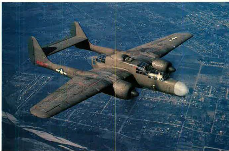
The US built only one night fighter during World War II: the P-61 Black Widow, Northrop's first major project. The first few off the production line, in 1943 (above), were painted olive drab and sported a gun turret atop the fuselage, but the aircraft soon received its trademark coat of black (opposite), and the turret was deleted after the first thirty-seven P-61As.
