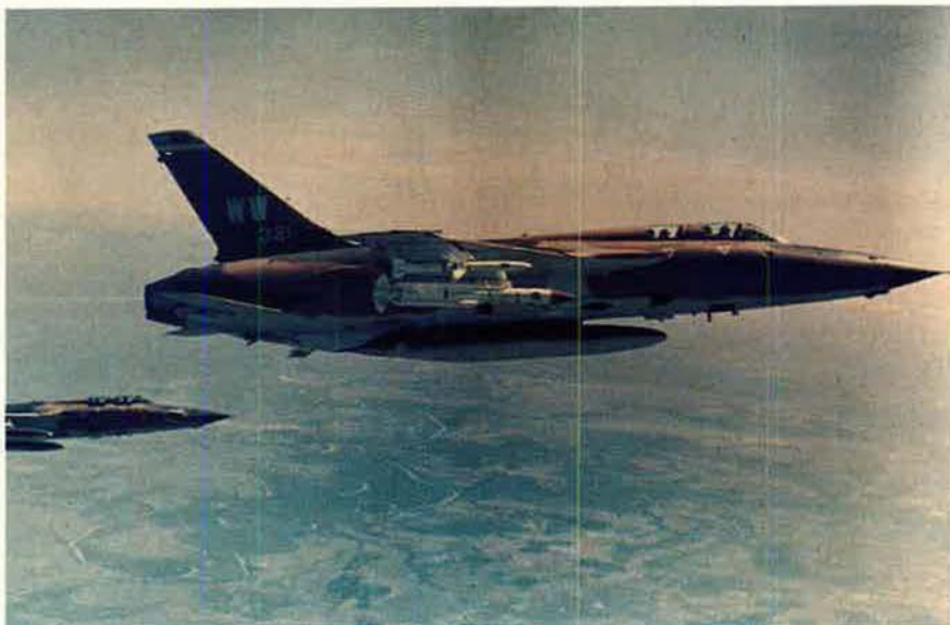
The electronic warfare technology that produced stunning results in the Gulf War had its beginnings in Vietnam. In response to the threat from surface-to-air missiles, the Air Force developed the Wild Weasels. Dedicated Weasel aircraft like this F-105G found SAM sites and took them out with AGM-45 Shrike missiles or AGM-78s.
