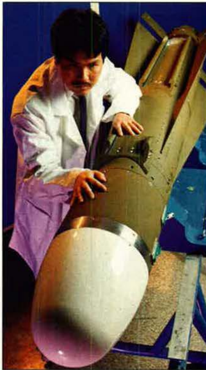
A Hughes Aircraft Co. engineer inspects a Maverick missile sporting a millimeter-wave, high-frequency radar seeker that allows the missile to acquire a target autonomously. The new Maverick, which will begin testing soon, is being developed under USAF's Balanced Technology Initiative.
