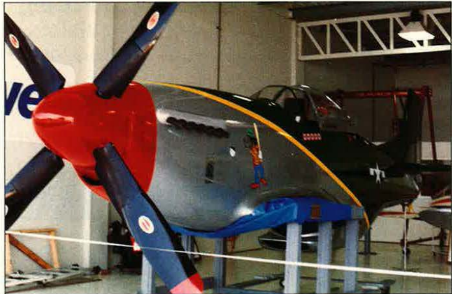
This all-composite, full-scale replica of the North American P-51 Mustang fighter weighs between 3,200 and 3,500 pounds empty; metal Mustangs can weigh from 7,800 to 11,000 pounds. The P-51 DH will be considerably faster than the original aircraft, with a top speed of around 500 mph.
