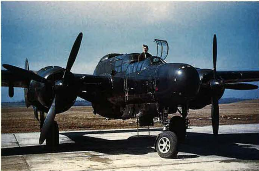
The P-61A was almost as large as and considerably faster than the North American B-25 medium bomber. Despite its size, the Black Widow could turn with most Allied fighters: In one formal contest with a P-47, the Widow came out on top. The P-61C, with its turbosupercharged engine, was even faster but came very late in the war.
