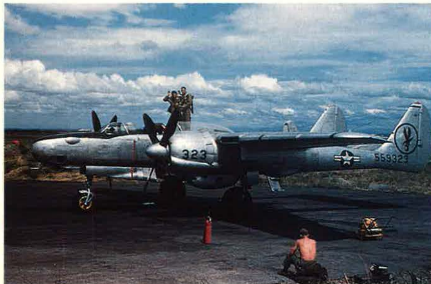
Only forty-one P-61Cs had been completed by the end of the war. With armament deleted and a new color scheme, the P-61 saw seven more years of service as the photoreconnaissance F-15A Reporter (above), redesignated RF-61C in 1948. A few P-61Bs became P-61Gs, modified for weather reconnaissance.
