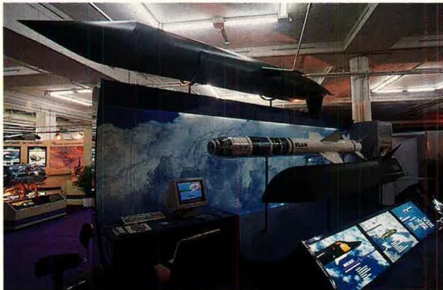
McDonnell Douglas's Advanced Cruise Missile (top) will improve the standoff lethality of US nuclear forces. Its Standoff Land-Attack Missile (center) was a great success in the Gulf War. Its Have Slick (bottom) has been successfully launched from an F-111E at subsonic and supersonic speeds, can deliver a unitary warhead or submunitions, and is being proposed for use on the multirole fighter of the future.
