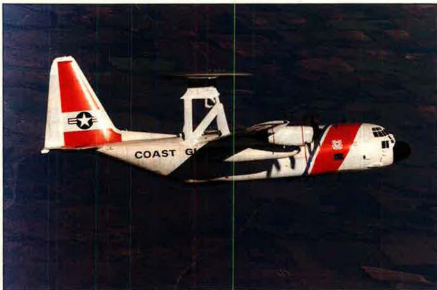
Flight testing of the first EC-130V Airborne Early Warning aircraft began at General Dynamics Fort Worth Division in late July. The company installed the Navy E-2C Hawkeye Airborne Early Warning Radar System into the long-range C-130 airframe to provide extended patrol capability for the US Coast Guard.
