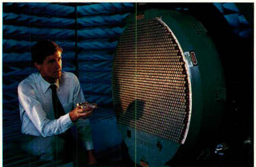
Electronic technologies are not being abandoned. Rome Laboratory is working on an indium phosphide-based technology that will increase electron mobility and resistance to radiation and electromagnetic interference—essential characteristics for such tactical devices as phased-array radar (above).
