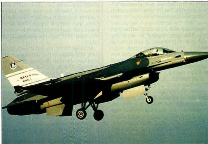
The Advanced Fighter Technology Integration (AFTI)/F-16 resumed flight testing in July after eighteen months of modifications. The program, managed by Air Force Systems Command's Aeronautical Systems Division, will include close air support testing at night in its current flight test phase, which will add several new capabilities to the aircraft, including FLIR and a night-vision helmet display system.
