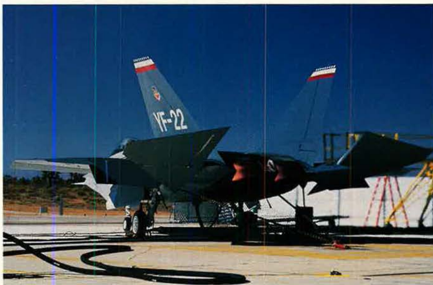
The F-22's Pratt & Whitney powerplant will have two-dimensional thrust-vectoring nozzles tailored to meet the Air Force's aerodynamic and low-observable requirements. They are able to vector thrust to a maximum of twenty degrees.
