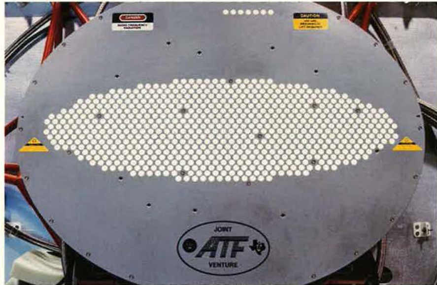
The F-22's radar features this active, electronically scanned array antenna that is designed to operate in about twenty-five modes and provides the aircraft with long-range target acquisition, target track, and fire-control capability.
