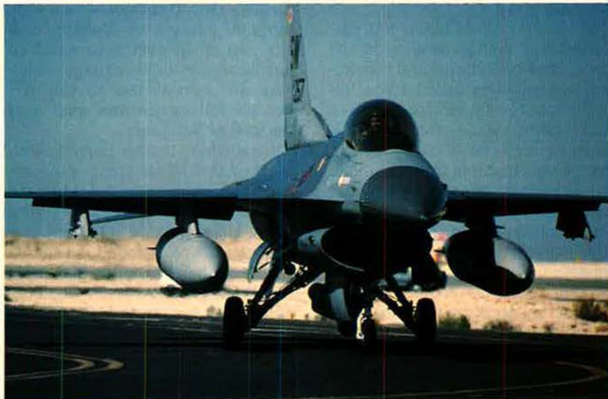
An F-16C returns from a Desert Storm mission with its bomb racks empty and an ALQ-119 ECM pod slung on its centerline. Air Force planes used assorted pods and internal jammers to great effect in fending off missiles and keeping losses very low.
