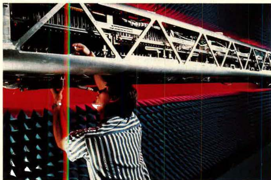
The heart of Joint STARS is its radar system, checked out above by technician Larry Mull in Grumman Corp.'s anechoic chamber in Melbourne, Fla. The radar was tested extensively in the chamber before being installed in the E-8A.
