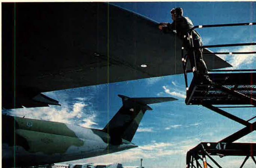
SSgt. Robert Blackwood of the 60th Operational Maintenance Squadron changes a left wing navigation light on a C-5A at Travis AFB, Calif. Airlift is a vital element of USAF's ability to deter war by transporting tactical air and ground forces over great distances for strategic purposes, as in Operation Desert Shield.
