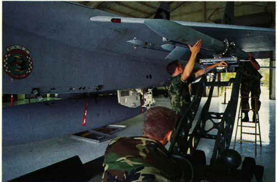
One major difference between the AIM-120 and the AIM-7 is that AMRAAM can also be carried on the LAU-128 underwing launch rail. Here, Sgt. Michael Hancock positions the jammer table under the rail while Sergeants Kennedy and Sharpe slide the missile off. The fins and wings will be added once the missile is secured.
