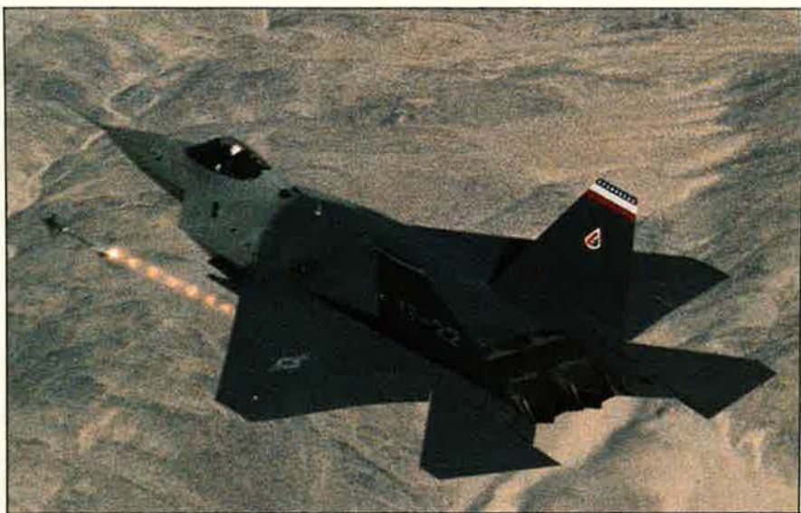
An AIM-9M Sidewinder air-to-air missile streaks away from the number two Lockheed/Boeing/General Dynamics YF-22 prototype during the single test conducted late last year, the first firing from either of the ATF designs. The missile was housed in the enclosed bay on the side of the aircraft's air intake.
