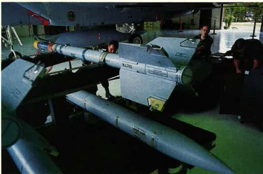
The combination of AMRAAM (bottom) and Sidewinder (top) seen on this load trailer at Eglin will be the primary weapons load for Air Force F-15s in the near future and for the ATF once it is fielded. Requirements call for the Air Force and Navy to buy 24,335 AMRAAMs, but this may be cut to 15,500 missiles.
