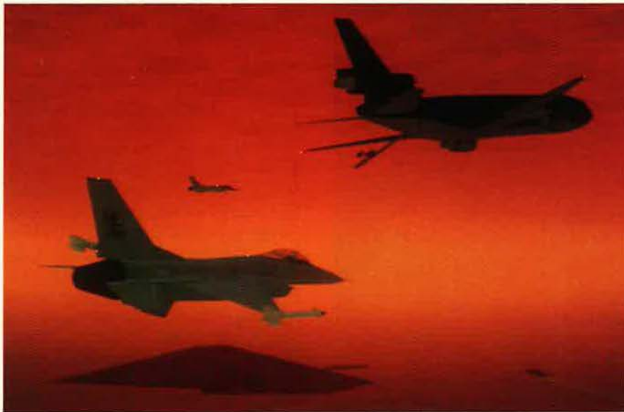
The T-1A simulator will make use of the Evans & Sutherland ESIG-500 image generator, with four infinity optics displays and a textured day/dusk/night capability. The ESIG-500 is also used on the Air Force's F-16 simulators and produces high-fidelity visual scenes like this F-16 about to refuel from a KC-10.
