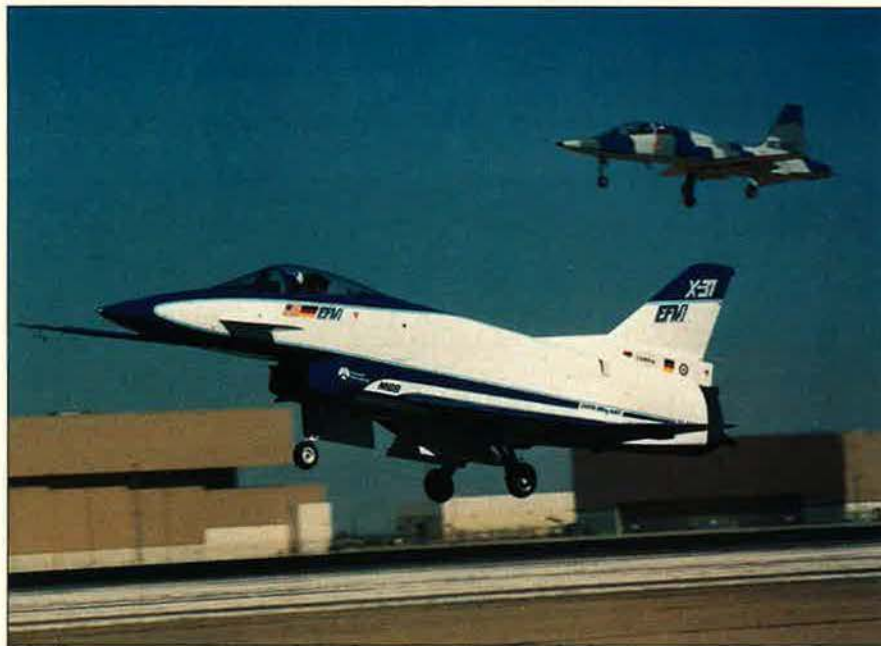
The Rockwell/MBB X-31A Enhanced Fighter Maneuverability aircraft comes in for a landing at Air Force Plant 42 in Palmdale, Calif., after its first flight October 11. Rockwell test pilot Ken Dyson was at the controls for the thirty-eight minute flight. The chase aircraft is a privately owned, civil registered Northrop T-38.
