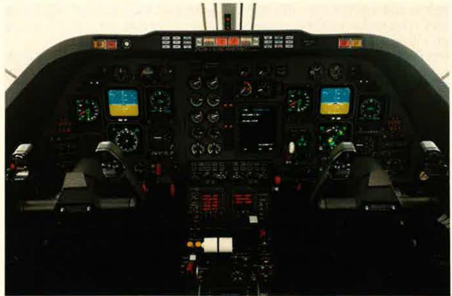
The Jayhawk and the T-1A simulator will make use of Collins's Pro Line 4 avionics package. The all-glass cockpit features side-by-side electronic primary flight display and multifunction display for student and instructor. It has an advanced map display capability and can show all nav aids, airports, and the active flight plan, as well as checklists, progress pages, and crew notes.
