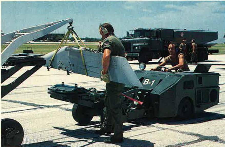
Falcon Baldwin '90 included an integrated combat turn of six F-16s. Accomplished quickly in 100-degree heat, the turn required the removal of 300-gallon centerline fuel tanks and, here, weapon pylons, as well as refueling and refitting the aircraft with AIM-9 Sidewinder air-to-air missiles.
