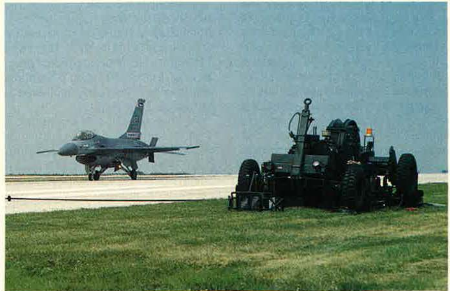
Prime BEEF engineering detachments also participated in the exercise. In addition to providing fire and rescue coverage, they set up this BAK-12 aircraft arresting system, which has been described as a "980-foot rubber band," at Baldwin Airport, Ill., to slow down and gently stop landing F-16s.
