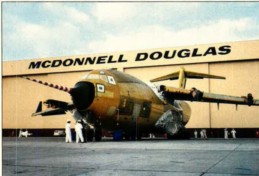
The first McDonnell Douglas C-17A airlifter came out of the production hangar at Long Beach, Calif., for the first time on September 16. The aircraft (here with an air data probe attached to its nose) will be pressure-tested at 11.04 pounds per square inch, about fifty percent higher than the pressure it is expected to encounter in an operational situation. The C-17A will fly by June 1991.
