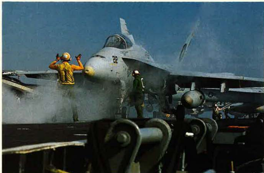
With the aid of a flight-deck director, an F/A-18 completes final lineup with the catapult in preparation for takeoff. Seconds later the pilot will remove his hands from the controls, because during the violent takeoff from the carrier deck, it is safer to leave the flying to the plane's computer and its built-in sensor.
