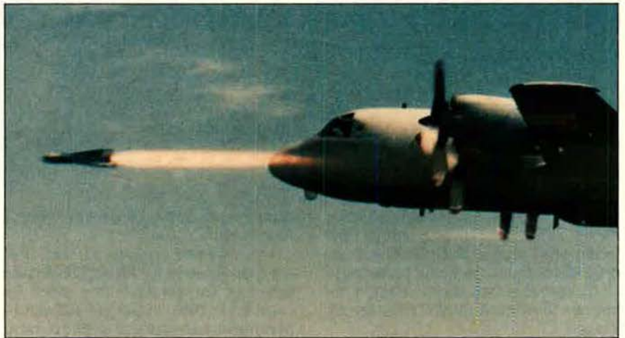
A Hughes AGM-65F Maverick missile is fired from a Navy P-3C Orion from the Naval Air Test Center, NAS Patuxent River, Md., in the first of a series of tests. The Navy's "F" version of the Maverick has a tracker fine-tuned to increase its effectiveness at sea.
