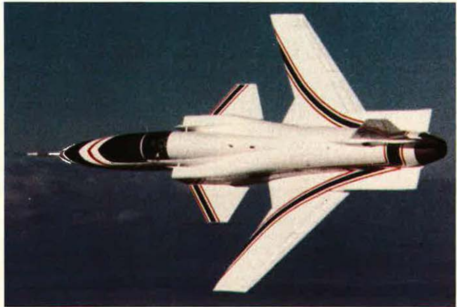
The Grumman-built X-29 Advanced Technology Demonstrator aircraft's forward-swept wings and advanced flight technologies allow unrestrained maneuvering at very high alpha. The second X-29 built achieved a sixty-six degree angle of attack.
