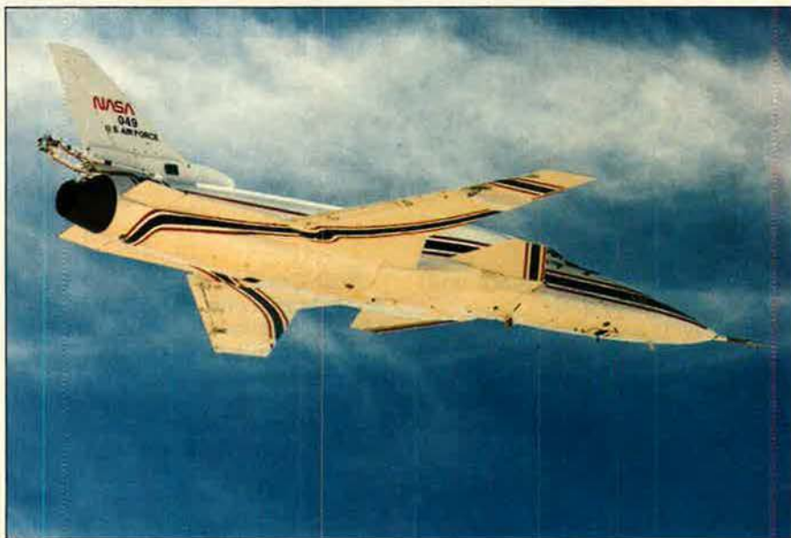
The number two Grumman X-29A Forward Swept Wing demonstrator has performed well in its high angle of attack test program now taking place at Edwards AFB, Calif. The aircraft is identical to the first X-29 except for some instrumentation changes and the addition of a fin-mounted spin recovery parachute. The X-29 high alpha test program is scheduled to continue into 1991.
