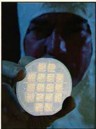
About the cover: This three-inch-wide gallium arsenide wafer contains sixteen complete radar transmit/receive cells. The assembly was fabricated by scientists at the Westinghouse Science & Technology Center in Pittsburgh.
