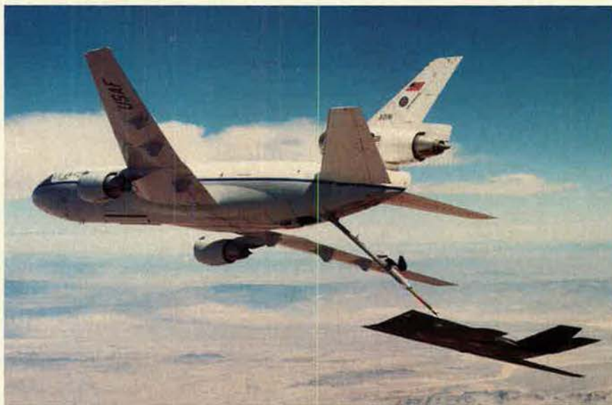
Any way you look at it, the F-117A is an unusual aircraft. Its design and development were also out of the ordinary. The F-117 is the first aircraft to exploit low-observable, or stealth, technology. Here, an F-117 tanks up in flight, just as those on their way to and from Panama did several times last December.
