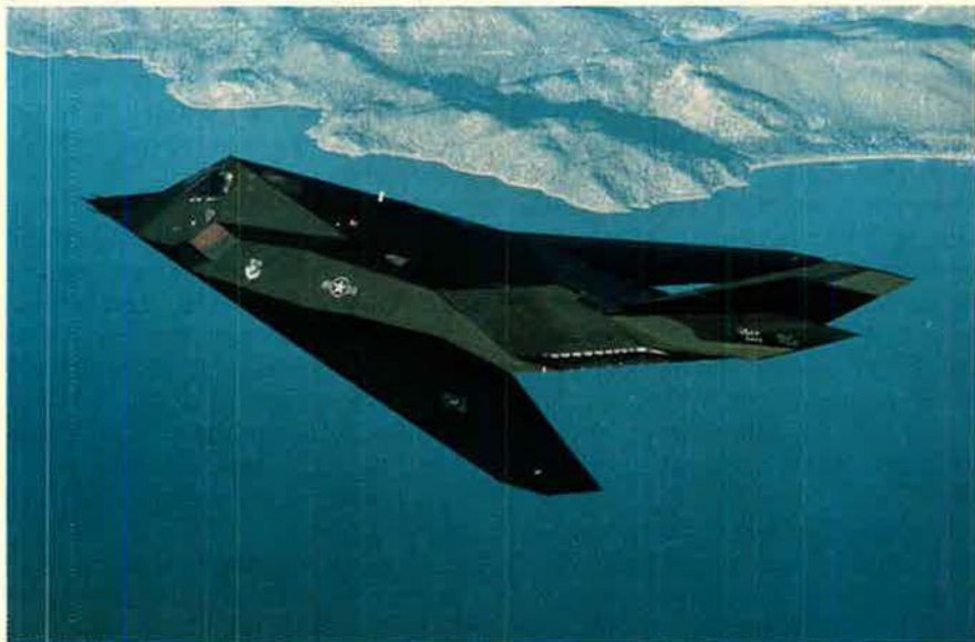
The faceted shape and radar-absorbent material covering give the F-117 its low radar cross section. The plane's exhaust (to the left of the movable ruddervators) can only be seen from above. Several measures, such as "burying" the engines and dispersing exhaust through baffles, are taken to reduce the efflux.
