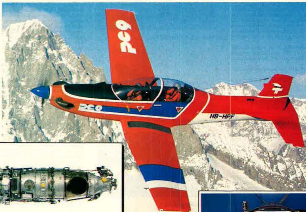
Latest technology 1,150 shp, flat rated to 950 shp, Pratt & Whitney PT6A-62 engine is fitted with electronic temperature and torque limiter.
