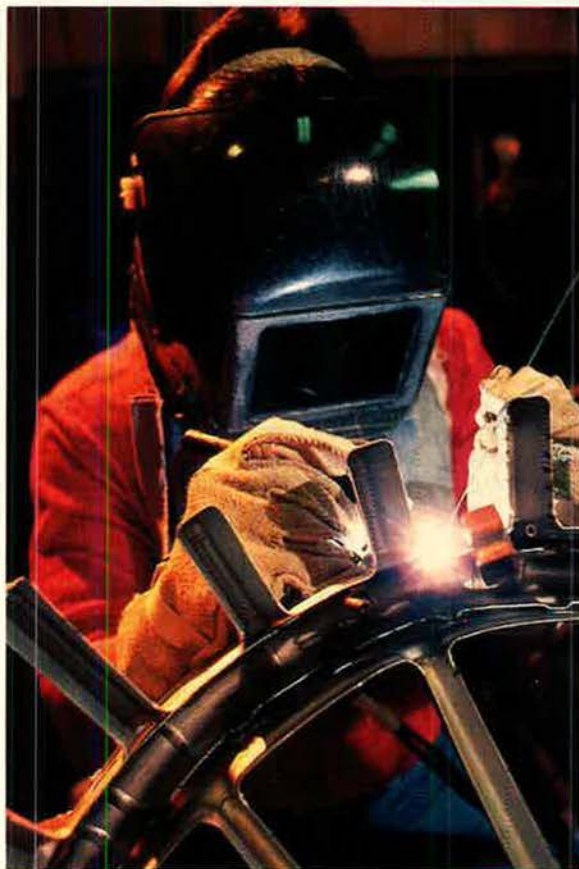
At San Antonio Air Logistics Center, Kelly AFB, Tex., Reynaldo Pentoja welds F100 engine parts. San Antonio ALC, system program manager for the Pratt & Whitney F100 engine, is one of AFLC's five air logistics centers whose programs keep the Air Force flying.
