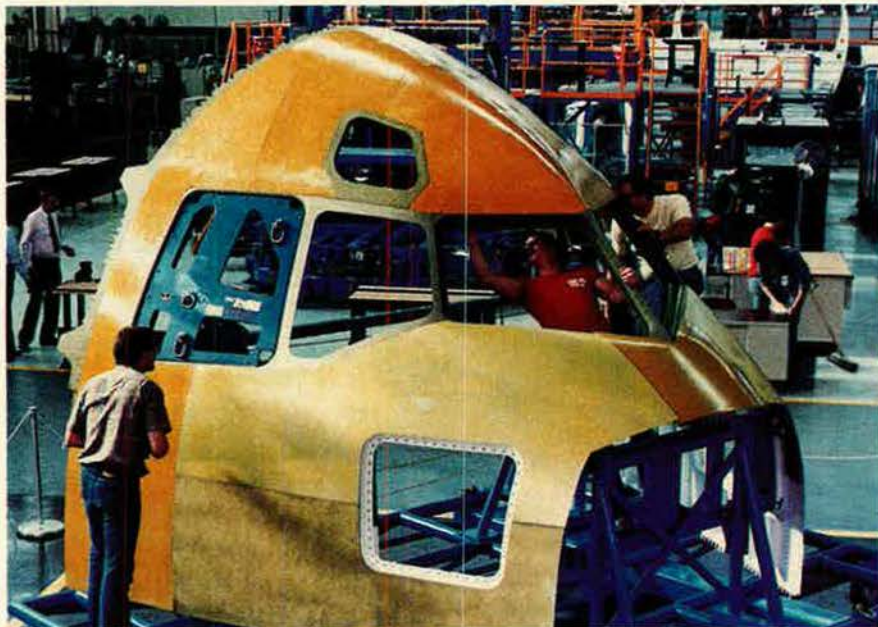
All of its parts and assemblies, like this upper cockpit section, are coming together, and the first McDonnell Douglas C-17A airlifter will be completed in Long Beach, Calif., late this year. The program has experienced some delays, and the plane's first flight is now expected to come in the middle of next year.
