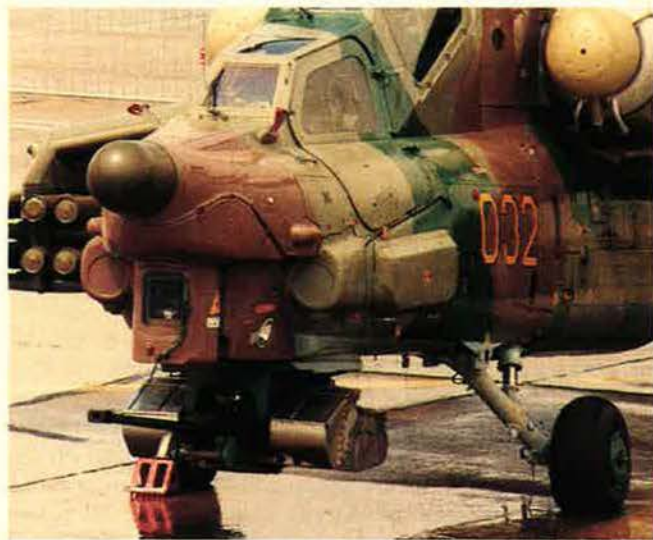
The Soviet Mi-28 "Havoc" is the Soviet counterpart to the US AH-64 Apache attack helicopter, and it is designed with front-line needs in mind. The undernose gun on the Mi-28 is also a standard weapon on many Soviet ground vehicles.
