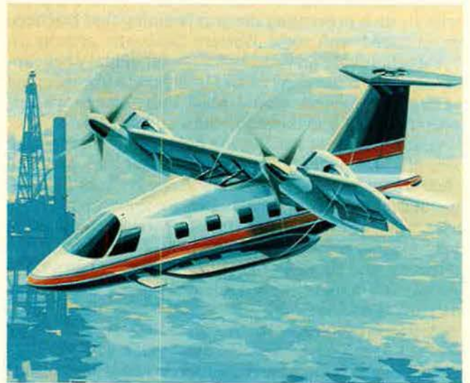
Japan plans first flight in 1992 of the Ishida TW-68, a tilt-wing transport similar to the V-22 Osprey. Less complex than the V-22, it will have maximum VTOL takeoff weight of only 12,500 pounds and seating for up to sixteen passengers.
