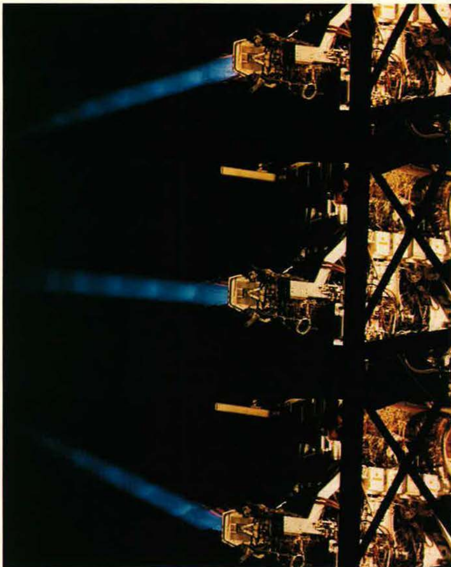
Although Pratt & Whitney has an advantage in vectored thrust work with the F-15 S/MTD program, General Electric has its own thrust-vectoring research program under way. This particular work is being done for the YF120-GE-100 Advanced Tactical Fighter Engine, but GE is also working on a possible thrust-vectoring nozzle to be retrofitted to the F-16 fleet.
