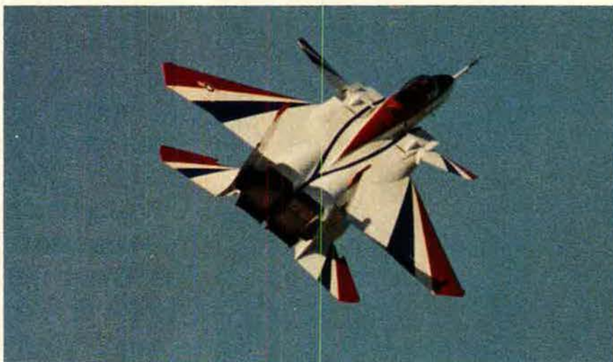
The integration that was required and the testing now going on with two-dimensional vectored-thrust nozzles on the Pratt & Whitney F100-PW-220 engines on the F-15 STOL/Maneuvering Technology Demonstrator (above) will have a direct impact on the YF119-PW-100 engine, a contender for the Advanced Tactical Fighter powerplant (right). The YF119 is undergoing sea-level testing at the company's plant in West Palm Beach, Fla.
