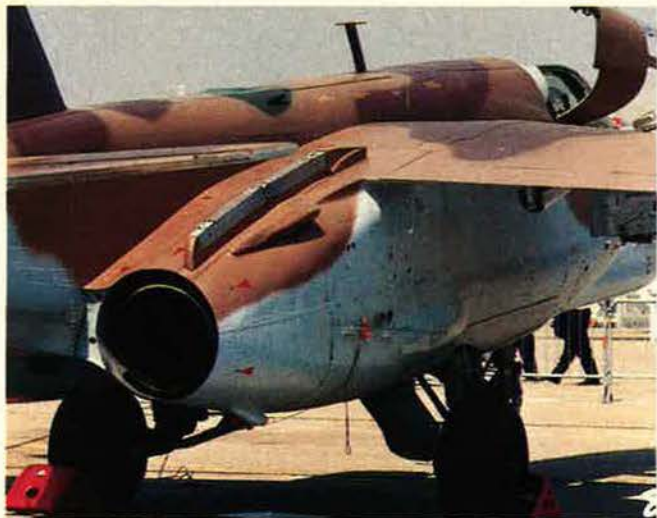
Flare containers on the engine nacelle of a Sukhoi Su-25 "Frogfoot," shown in Paris. The Su-25 has massive wings, is highly maneuverable, and can operate from short, rough, unpaved air strips.
