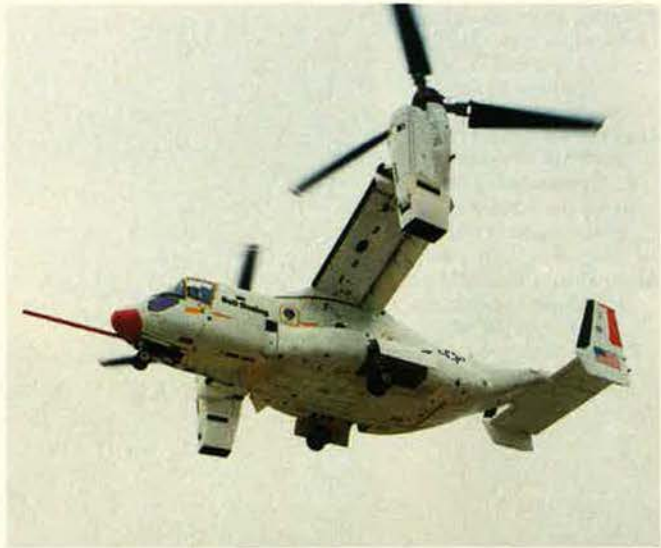
The US-built V-22 Osprey is much larger than Japan's VTOL transport entry, the TW-68. The Osprey has a maximum VTOL takeoff weight of 47,500 pounds and seats twenty-four passengers. Its pivoting wings and tilting rotor pods enable it to meet shipboard stowage requirements.
