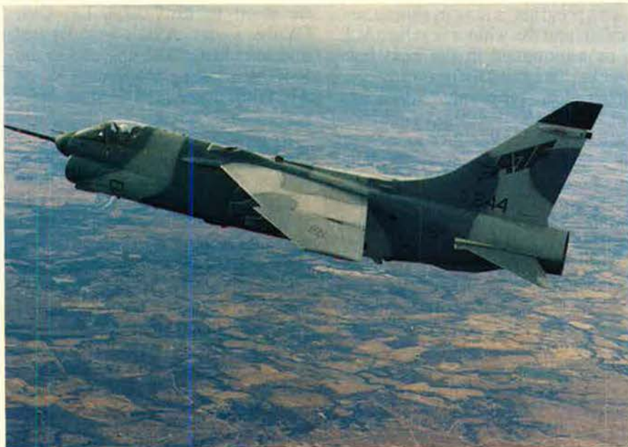
The first LTV YA-7F flew late last year and will be joined by a second aircraft next month. The two YA-7Fs (greatly modified A-7Ds) will undergo a ten-month flight-test program to verify design and performance characteristics. This is the first YA-7F on its initial flight from the company's Dallas, Tex., facility last November.
