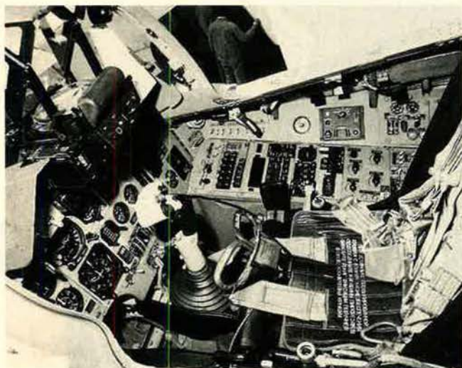
Instrumentation in the cockpit (above) of the Sukhoi Su-27 "Flanker," seen at the Paris Air Show last summer, is of 1960s vintage, and the airframe (right) contains little composite material. Still, the high quality of today's Su-27 and plans to build improved versions permit the USSR to move directly into development of a Soviet equivalent of USAF's Advanced Tactical Fighter.
