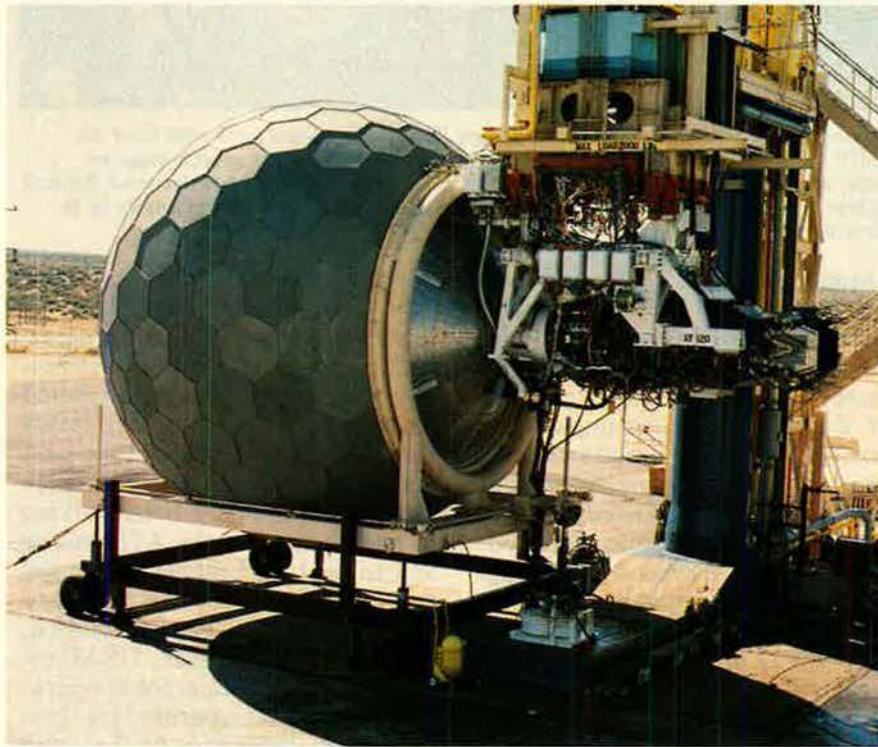
The two competing ATF engine companies are taking different approaches to meet USAF's stringent requirements for fighter engines. General Electric took the "variable cycle" approach with its YF120-GE-100 (shown here). The engine should have the economy of a turbofan in low speeds and the performance of a turbojet in the supersonic regime.
