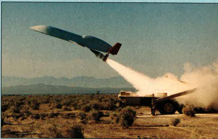
Booster-assisted launch of a Teledyne Ryan Model 324 Scarab RPV
