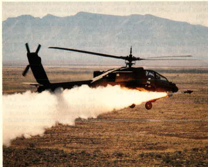
The Army is intent on arming its attack helicopters with air-to-air missiles to enable them to defend against Soviet helicopters similarly armed. The top picture shows a Stinger mounted on an Apache alongside ground-attack missiles. In the photo directly above, an Apache launches a Sidewinder during a recent test.
