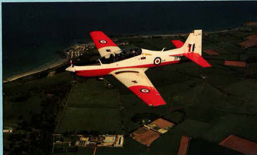
The Shorts Tucano T. Mk 1 is replacing the Jet Provost as the Royal Air Force's standard basic trainer
