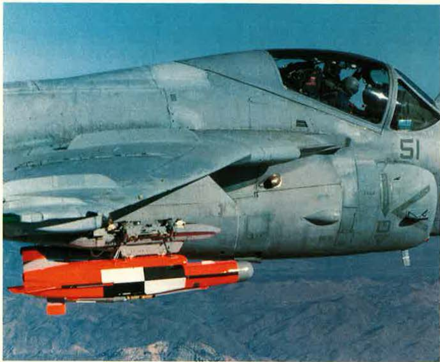
A Northrop Tacit Rainbow remotely piloted, radar-homing "loitering missile" takes to the air for a test aboard a Navy A-6. Such unmanned airborne vehicles (UAVs) seem to be catching on in all the military services as the means of augmenting manned aircraft.
