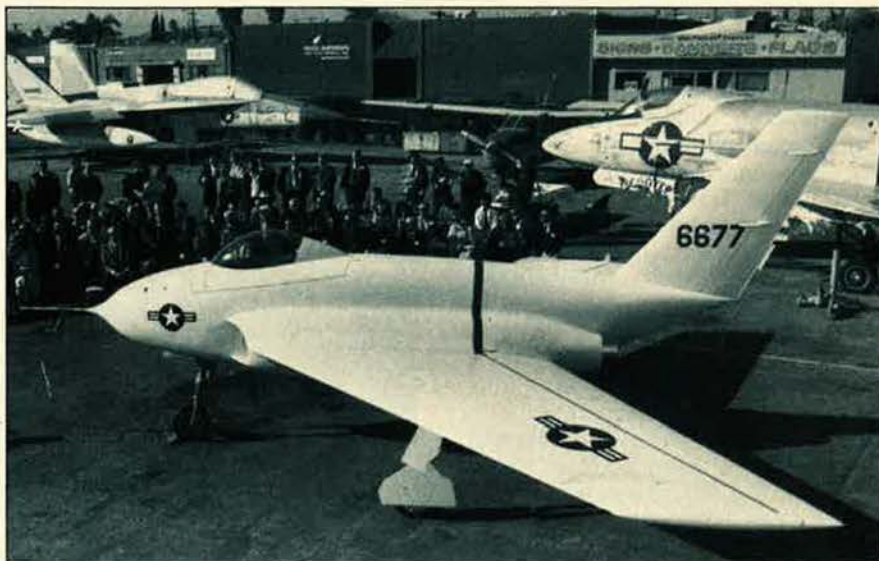
The Northrop X-4 Bantam was recently rolled out after being restored. The X-4, designed in the 1940s to test "compressibility" effects in the transonic regime, will be displayed at the Air Force Museum at Wright-Patterson AFB, Ohio (see item).
