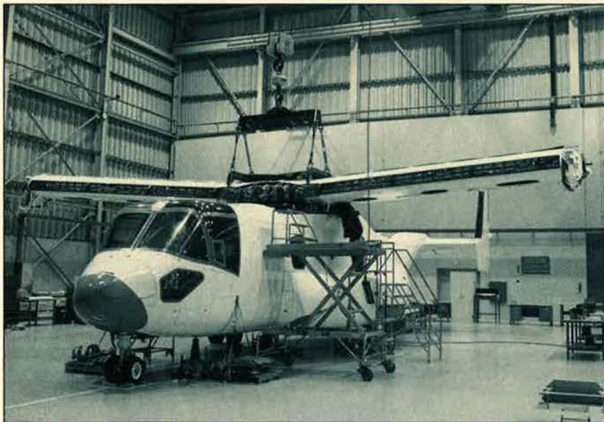
It's looking more and more like an actual airplane. The wings of the first Bell-Boeing V-22 Osprey flight-test article were mated to the fuselage in early February at Bell's Arlington, Tex., facility. The procedure took less than twenty-four hours. The first flight is set for early summer.
