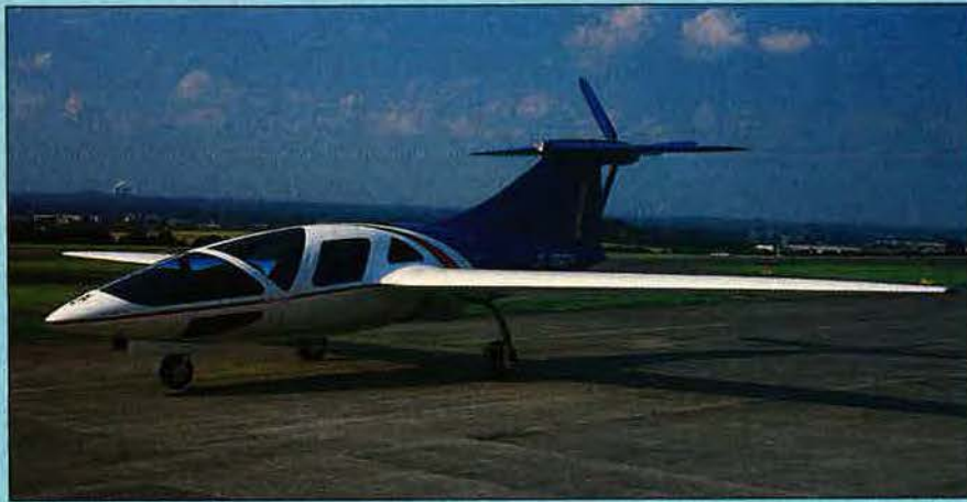
The Colani/Composite Engineering Cormoran CCE-208 five-seat all-composites light aircraft in latest configuration
