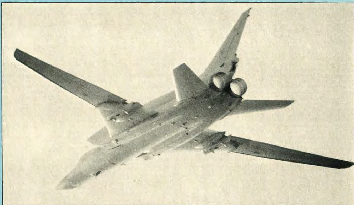
This new photograph of 'Backfire-C', in a hurry to get away from the inquisitive interceptor, shows the wedge intakes and underwing pylons for 'Kitchen' missiles
