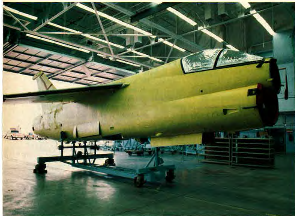
An A-7D ground-attack aircraft is being stripped down at LTV's Texas plant while taking shape as the first prototype YA-7F. USAF hopes to build such enlarged and "enhanced" A-7s for interim duty as CAS aircraft in support of the Army well into the 1990s.
