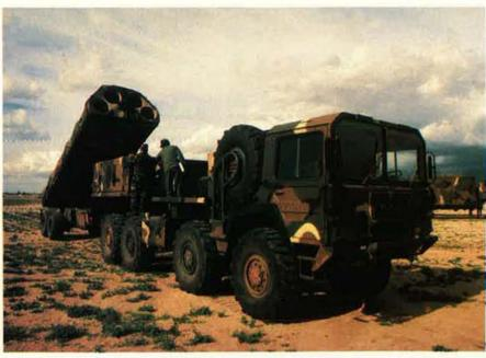
One of USAFE's unique missions is that of operations with the BGM-109 Tomahawk ground-launched cruise missile, or GLCM. USAFE will eventually have six operational wings of these weapons. This is one of the transporter/erectors that can carry four missiles.
