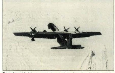
This Lockheed LC-130F was recently dug out of "deep freeze" on McMurdo Sound in Antarctica. After an aborted takeoff sixteen years ago, the plane was abandoned and became covered with ice and snow, leaving exposed only the top three feet of its thirty-eight-foot-high stabilizer. The plane was found to be structurally sound and will likely be flown out after a few weeks of field repair.
