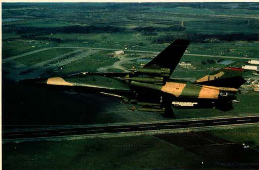
An F-111F from the 48th TFW at RAF Lakenheath, UK, banks away. This F-111 is carrying four Paveway II laser-guided weapons and has its Pave Tack laser designator deployed under the forward fuselage. F-111s with precision-guided weapons will be used for knocking out critical enemy targets far behind enemy lines.
