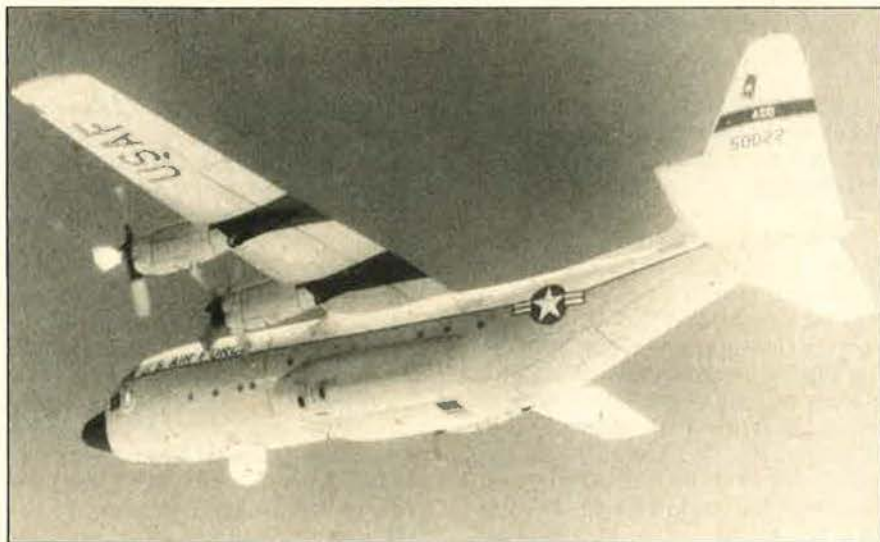
This modified C-130 is carrying out the first flight test of the Airborne Seeker Evaluation Test System (ASETS). ASETS extends forty inches below the C-130 fuselage and can evaluate several seekers or sensors at the same time. (USAF photo by SMSgt. William L. Patterson)
