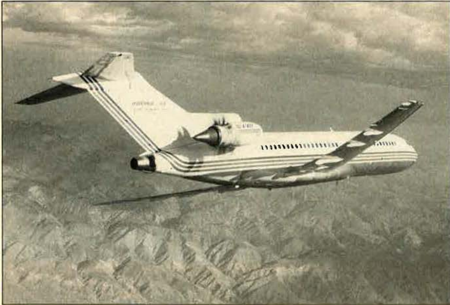
The first ultra-high-bypass turbofan engine was successfully flown on this modified Boeing 727 on August 20. The aircraft reached speeds of 300 knots and altitudes as high as 21,000 feet during its sixty-seven-minute flight. The General Electric proof-of-concept unducted fan engine has the potential to revolutionize commercial aviation in the 1990s.
