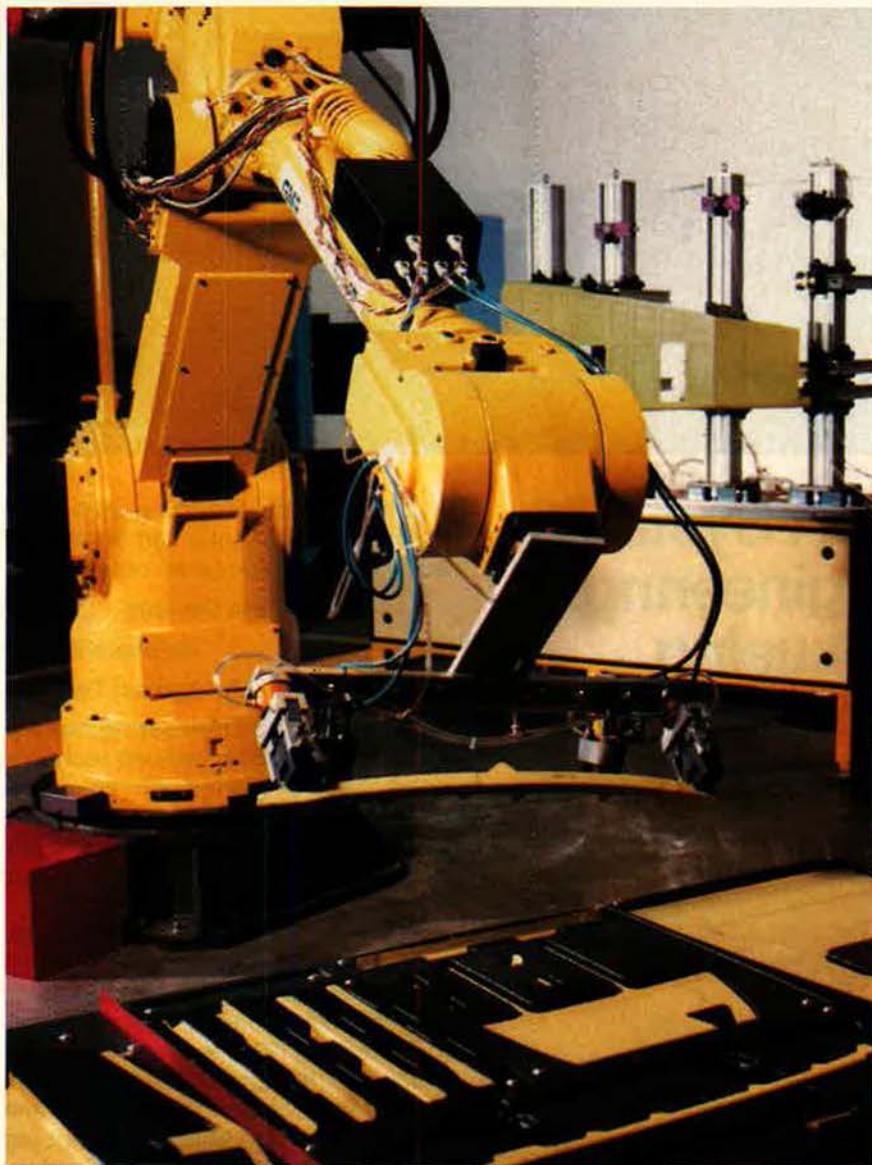
A Rohr Industries robot handles airframe components in the company's new flexible assembly subsystems (FAS) facility. Rohr is a leader among the growing number of subcontractors participating in USAF manufacturing modernization programs.
