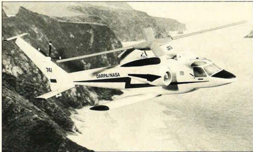
The X-Wing concept combines the advantages of helicopters and fixed-wing aircraft into one airframe. While this is just a model of the X-Wing attached to the Army/NASA Rotor Systems Research Aircraft (RSRA), the real X-Wing was rolled out on August 19 and should be flying in October.
