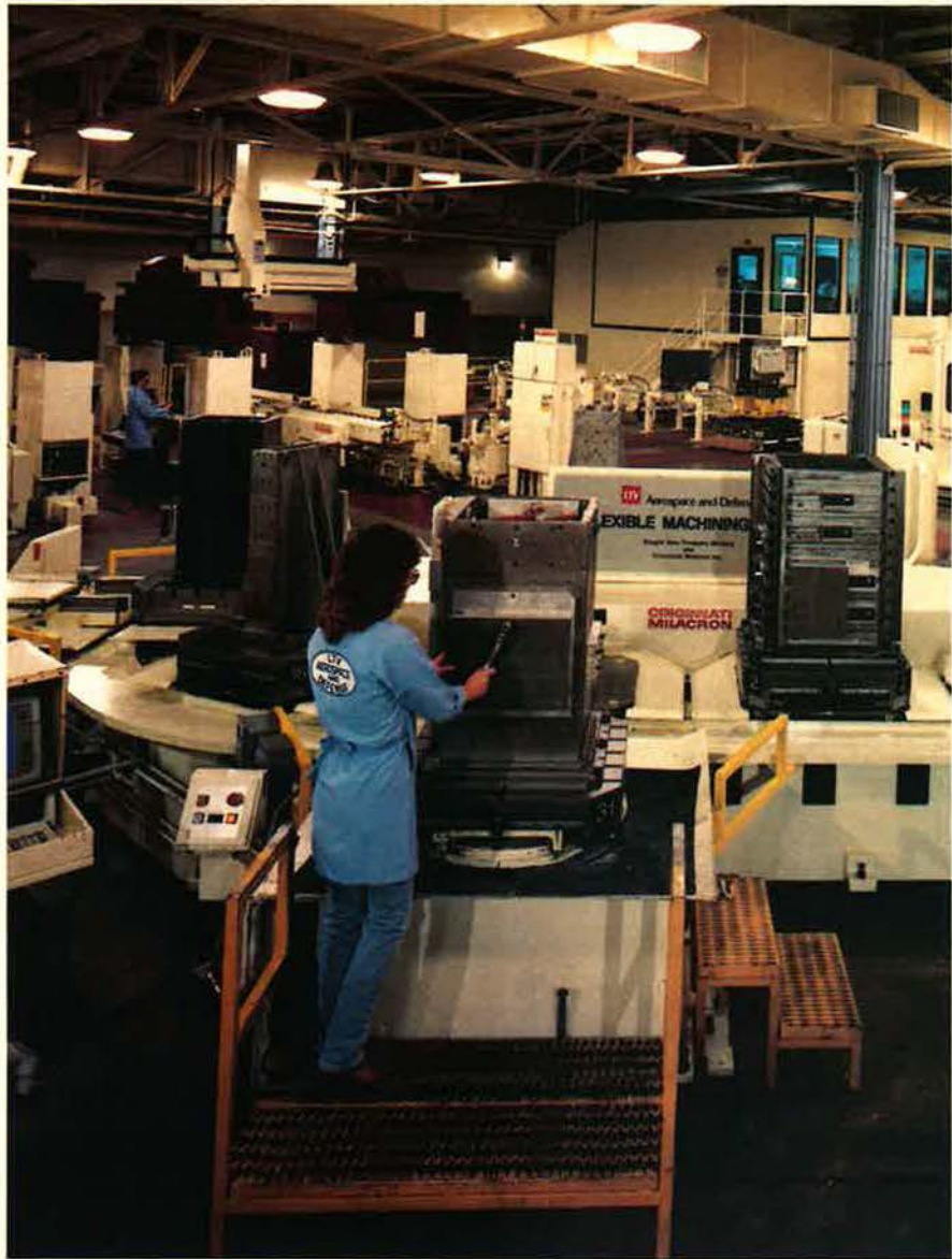
Vought Aero Products Division's highly automated flexible machining cell (FMC) is said to be the most sophisticated computer-controlled facility of its kind in the world. It machines 541 parts for the B-1B bomber.
