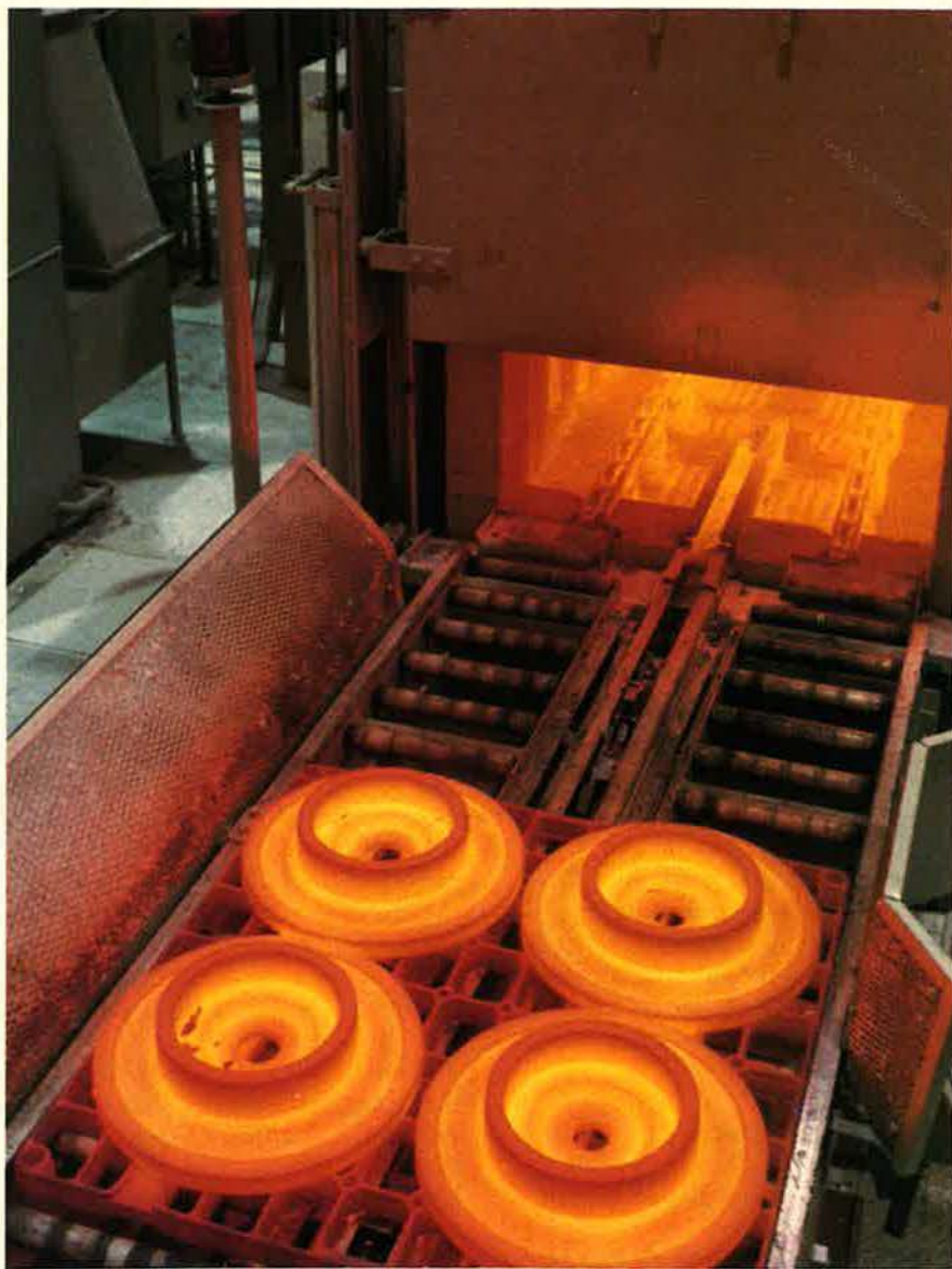
Forged engine disks emerge from a furnace in the heat-treating work cell at Pratt & Whitney's new plant in Georgia. USAF TechMod seed money helped to stimulate P&W's construction of the up-to-date facility.
