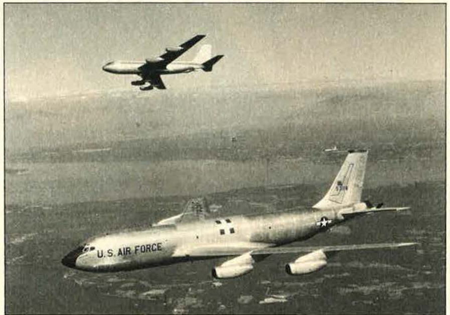
For the past thirty years, the Boeing KC-135 Stratotanker has been filling the tanks of military airplanes all over the world. This picture shows the very first KC-135A (serial number 55-3118, the City of Renton) with the Model 367-80, its progenitor, peeling off. 55-3118 is still flying with TAC as an EC-135K.
