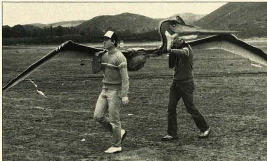
Technicians walk the model Quetzalcoatlus northropi, or QN for short, to its launching trolley before one of the pterodactyl's flights in January. The QN is the first man-made device to be stabilized by flapping wings.
