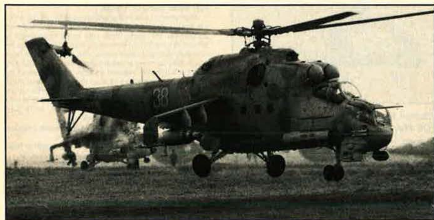
Mil Mi-24 (NATO 'Hind-E') with twin-barrel cannon instead of nose turret (Camera Press)
