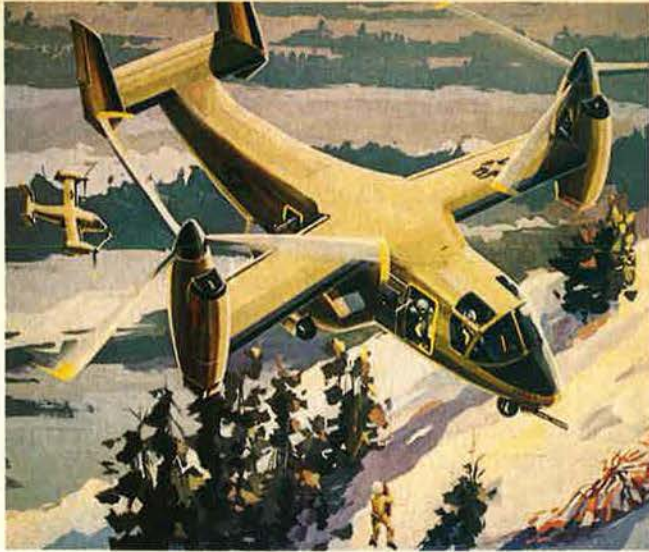
The Bell-Boeing CV-22 Osprey tilt-rotor design, here shown in artist's concept, will complement the MC-130s in deep "infiltration and exfiltration" missions and will reduce shortfalls in SOF airlift.
