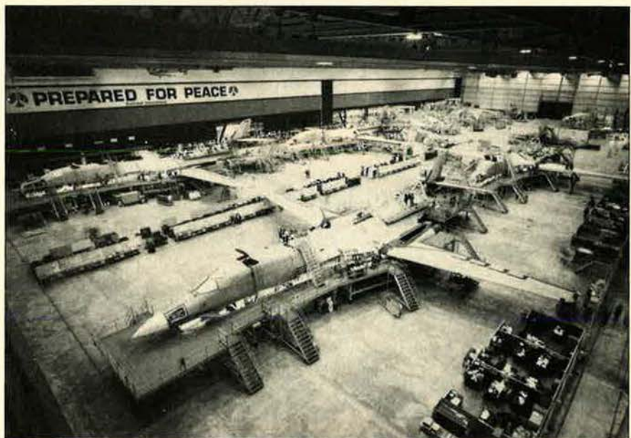
The Rockwell International plant at Palmdale, Calif., is busy as B-1B production swings into high gear. This photo shows seven aircraft (numbers fifteen to twenty-one) being fabricated in the final assembly building.
