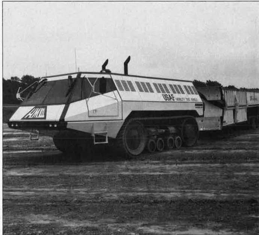
The full-scale hard mobile launcher test vehicle for the small ICBM (or "Midgetman") developed by Martin Marietta and Caterpillar maneuvers over a test course in Peoria, Ill. The Martin Marietta/Caterpillar design will be in a competitive "runoff" with a launcher developed by Boeing and Goodyear over the next year.
