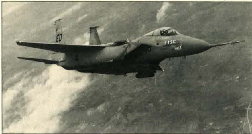
An F-15C from Edwards AFB tests the navigation pod (under left intake) of the Air Force's Low-Altitude Navigation and Targeting Infrared for Night (LANTIRN) system. This test is an important step in the development of the F-15E dual-role fighter.
