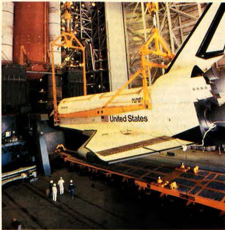
The Orbiter Enterprise inside Vandenberg AFB's Shuttle Assembly Building, where Discovery will be mated with its solid rocket boosters and its external tank. The boosters are 149 feet high, twelve feet in diameter, weigh about 1,300,000 pounds each, and are assembled at Vandenberg.
