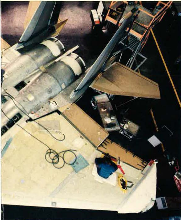
Workers at McDonnell Douglas Corp.'s St. Louis, Mo., plant splice the center and aft fuselage sections of an F-15 fighter. McDonnell Douglas has made major capital investments in plants and equipment for fixed-wing aircraft, helicopters, semiconductors, and simulators in order to maintain its competitive position.
