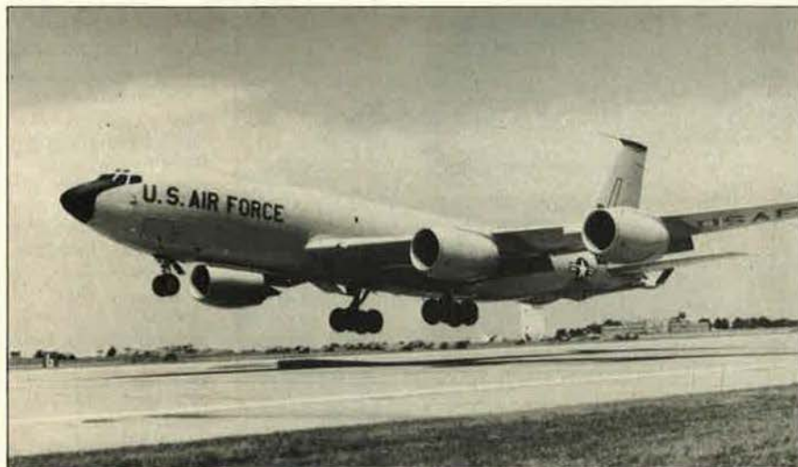
The Boeing Military Airplane Co. has received a contract to continue installing CFM56 engines on KC-135R tankers. With the newer, quieter, more fuel-efficient engines, Boeing claims that two KC-135Rs can do the work of three KC-135As.
