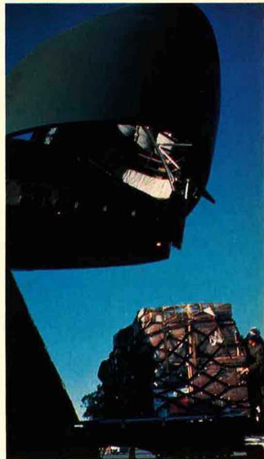
A C-5 Galaxy, largest operational aircraft in the world, opens its visor-type hinged nose to allow loading of palletized cargo for a long-range deployment. Loading is facilitated by adjusting the height of the cargo floor, which is normally at truck-bed level.
