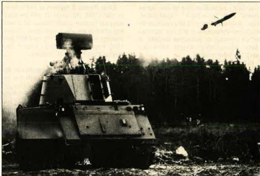
A Bofors RBS 70 low-level air defense missile is fired from a proposed turret-mounted launcher being considered for purchase by Canada. The RBS 70, which is laser-guided and has a US-made IFF system, has replaced the US Redeye in the Australian Army.
