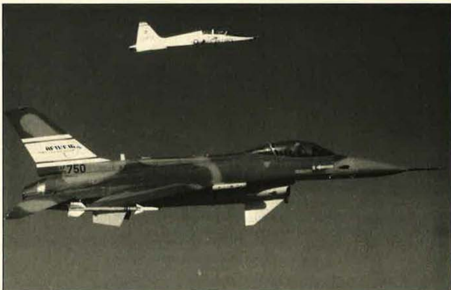
The USAF Advanced Fighter Technology Integration AFTI/F-16, equipped with a new forward-looking infrared (FLIR) tracking system, flies with a T-38 chase plane over Edwards AFB, Calif. The FLIR is attached at the wing root.
