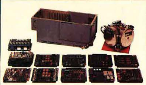
Litton LN-93 RLG INU for Standard Navigation The advanced technology LN-93 will meet the latest USAF Standard Inertial Navigation Unit requirement.
