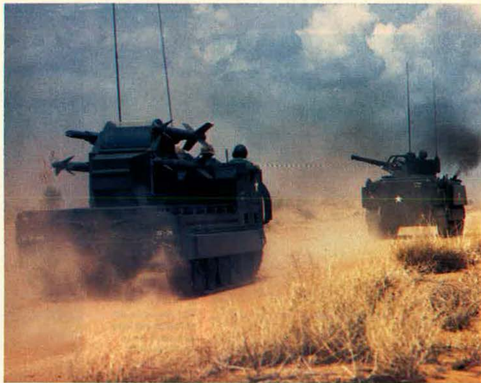
The highly mobile, air-transportable Chaparral allows for maximum flexibility of ground-based air defenses. The self-propelled version of Chaparral pictured in the foreground carries four modified Sidewinder missiles on launch rails and eight additional missiles in internal storage compartments.
