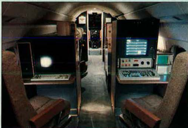
LEFT: SRA-1, mid-cabin, looking forward, with mission director's display at left, SLAMMR console at right. RIGHT: Inside the SRA-1 demonstrator: Lorop camera in right foreground
