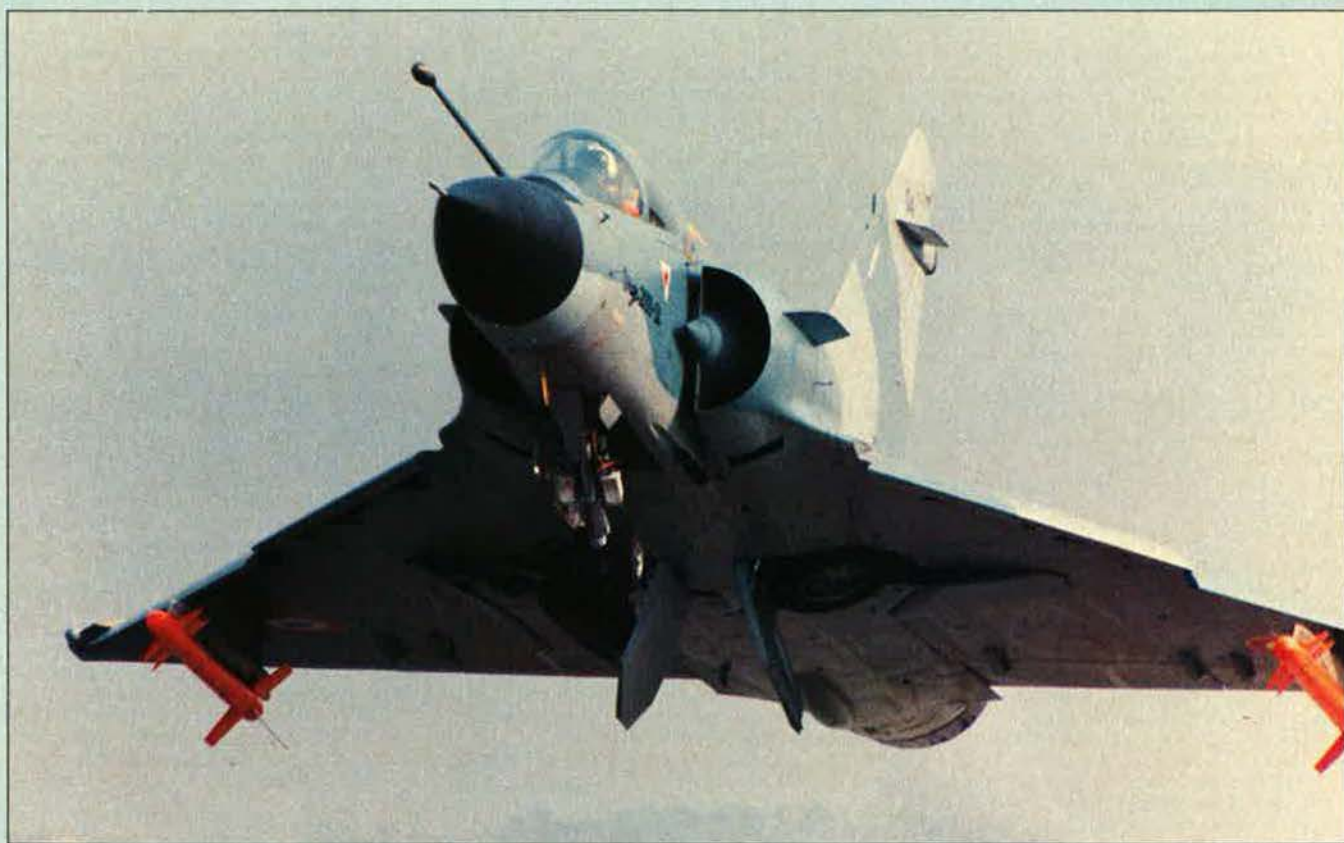
Take-off shot of Mirage 2000C1, with flight refuelling probe and underwing Magic missiles
