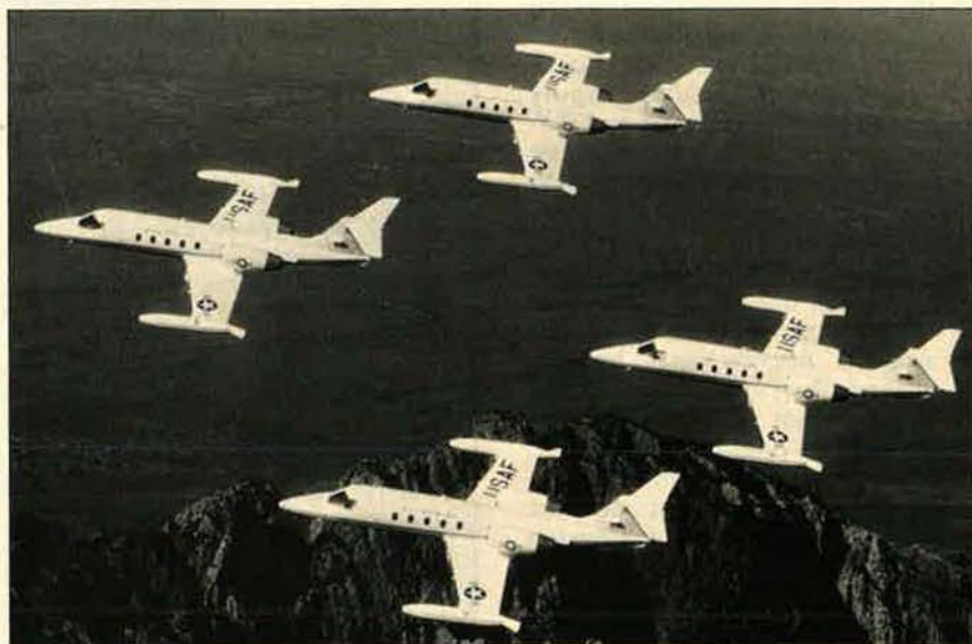
The Gates Learjet C-21A, replacement for the CT-39 Sabreliner, is part of USAF's new operational support aircraft fleet. Here, four are seen in diamond formation.
