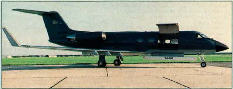
Gulfstream SRA-1 demonstrator with underbelly SLAMMR (side looking airborne multi-mode radar) pod
