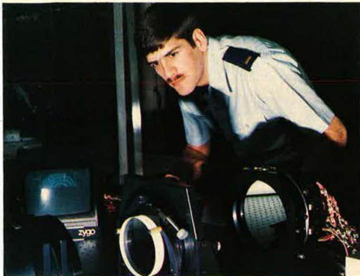
A Rome engineer checks adaptive mirrors for space-based electro-optical surveillance programs. (USAF photo by Larry Rocco)
