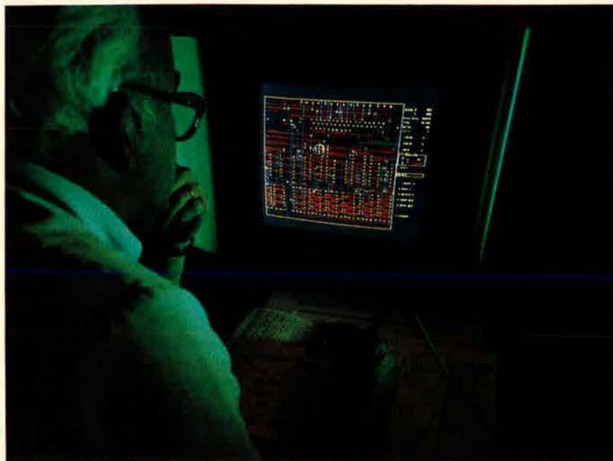
Allied Bendix Aerospace designer Bill Lins uses computer-aided design to transition circuits to the large-scale-integration (LSI) packaging required for the Mark XV IFF system, which must be made to fit into the space allocated for the current Mark XII system. (Allied Bendix photo by Bill Perich)
