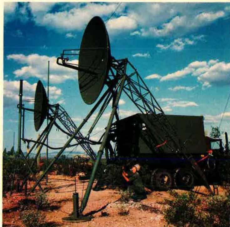
The TRC-170 sends more accurate messages over longer distances than do current battlefield radios. (USAF photo by Larry Rocco)
