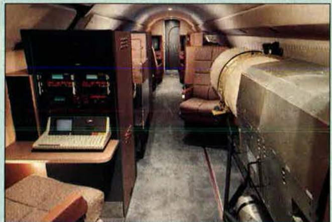
LEFT: SRA-1, mid-cabin, looking forward, with mission director's display at left, SLAMMR console at right. RIGHT: Inside the SRA-1 demonstrator: Lorop camera in right foreground
