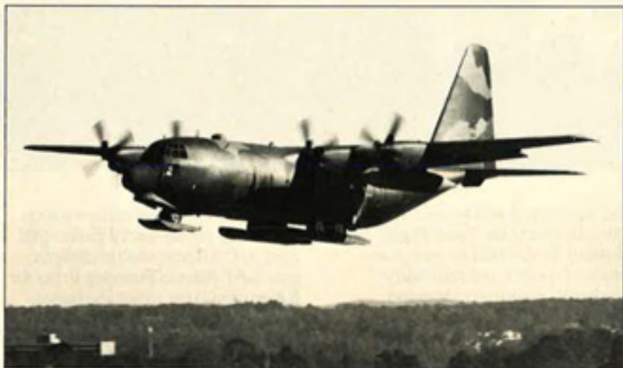
One of four new Lockheed LC-130H Hercules aircraft, largest in the world to be outfitted with skis, demonstrates the Lockheed ski-and-wheel system, which enables operation from both paved and snow or ice runways.
