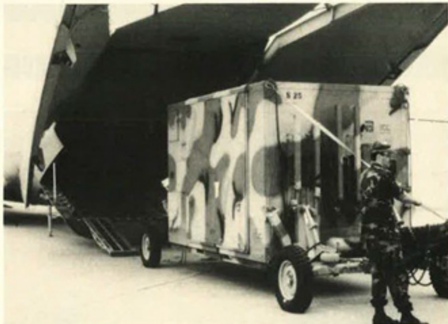
An electronic equipment van is loaded aboard a C-141 as part of an ESC unit deployment for a field exercise. Such mobile units create hostile electronic warfare conditions to test US forces' countervailing capabilities.
