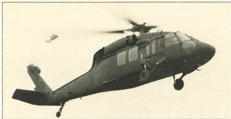
The Army, with USAF funding, is testing a new version of the Sikorsky UH-60A Black Hawk helicopter that has a composite rear fuselage instead of the standard metal fuselage. USAF will use the Black Hawk for search and rescue.
