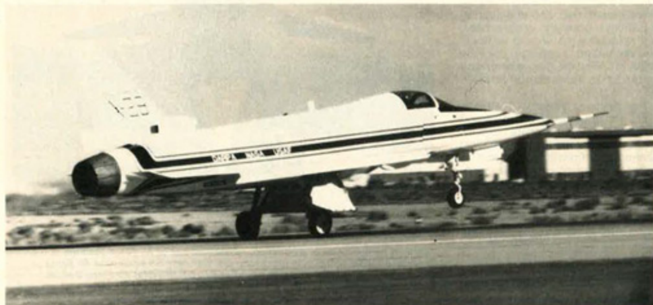
The first X-29 advanced technology demonstrator aircraft, featuring forward-swept wings, takes flight at Edwards AFB, Calif. AFSC teamed with Grumman Aerospace Corp. and the Defense Advanced Research Projects Agency in developing and building two X-29 test-bed aircraft.
