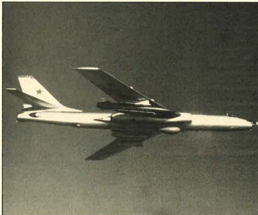
AS-6 'Kingfish' missile on Tupolev Tu-16 (NATO 'Badger-G' modified) (Swedish Air Force)
