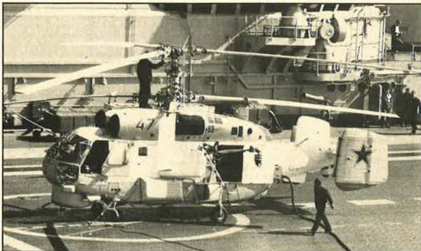
SAR and plane guard version of Kamov Ka-27 (NATO 'Helix-A') (Royal Navy)
