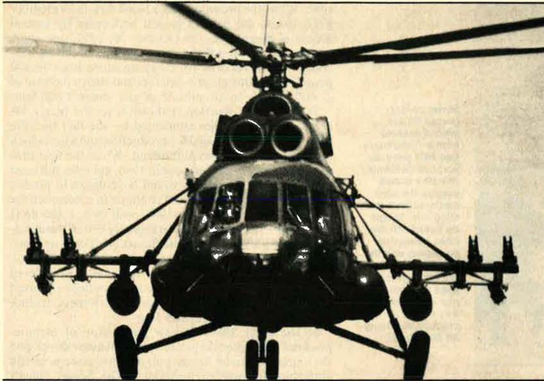
Mi-8 Hip-E assault helicopter bears down at point-blank range. About 10,000 of these choppers have been produced, in keeping with Soviet development and refinement of airmobile assault concepts. The Mi-17, an updated variant of the Mi-8, is now entering quantity production.
