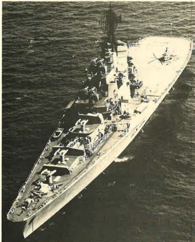
Soviet Moskva helicopter carrier at anchor. Aft, Moskva and her sister ship Leningrad each carry up to fourteen Ka-25 Hormone antisubmarine warfare helicopters and a utility variant. Forward, each is outfitted and armed as a missile cruiser, deploying anti-aircraft and ASW weapons.
