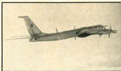
Tupolev Tu-142 (NATO 'Bear-F') with MAD tail 'sting' (Royal Norwegian Air Force)
