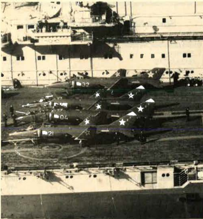
Yak-38 Forger VTOL fighters arrayed with wings folded aboard the Kiev. The 901-foot Kiev-class carriers also feature anti-air/anti-surface/anti-submarine weapons similar to those on large Soviet missile cruisers, and can fight their own way out of trouble.
