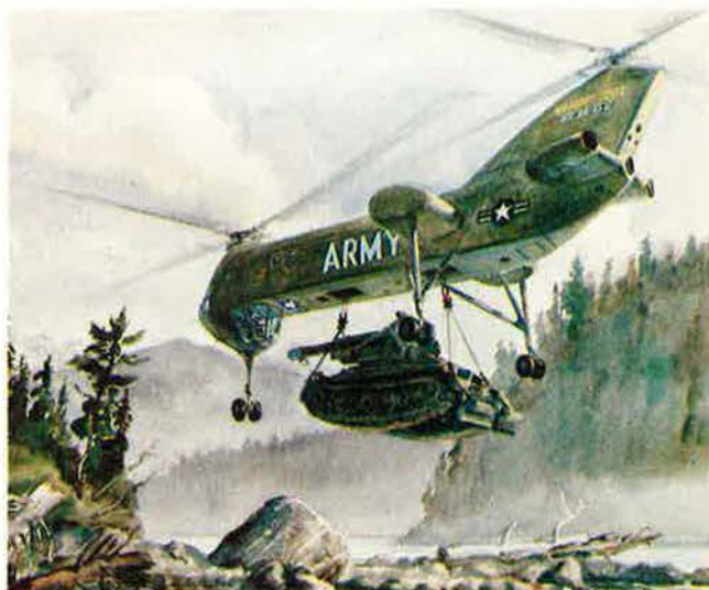
Heavy-lift helicopters might be the best method of supplying combat areas having vulnerable or cratered runways. Welcome news in 1984 was that Boeing is to complete and test the XCH-62, with a lift capability of thirty-five tons, after the program was shelved for nearly ten years.
