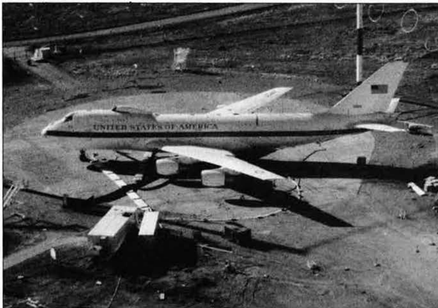
The E-4B Advanced Airborne Command Post is designed to survive in nuclear war, with communications, electronics, and display systems hardened against electromagnetic pulse (EMP) and transient radiation effects on electronics (TREE).
