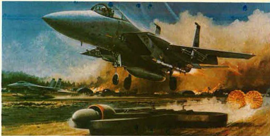
Artist's rendering shows how fighter aircraft may someday take off from air-cushioned platforms that propel them to rotation speed over bomb-damaged runways.
