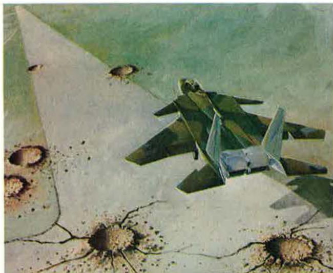
Advanced technology F-15, with foreplanes and vectoring nozzles, will operate from 1,500-foot strips.
