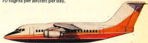
British Aerospace 146 – powered by US-built fanjets – will bring ultra-quiet, wide-body services to commuter and feeder routes from 1982.
