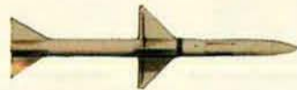
Sky Flash – the Western World's most advanced radar-guided, all-weather, air-to-air missile, based on the Raytheon Sparrow.
