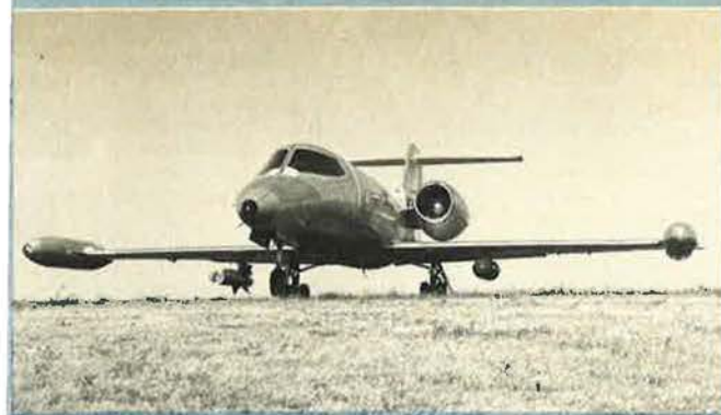
Above: Special missions Learjet 35A, with Hayes International TGX-1 visually-augmented target under starboard wing and Interdyne Corporation LJ-25 sonobuoy/flare dispenser under port wing. Right: Loading LUU-2B flares into the Learjet's LJ-25 dispenser
