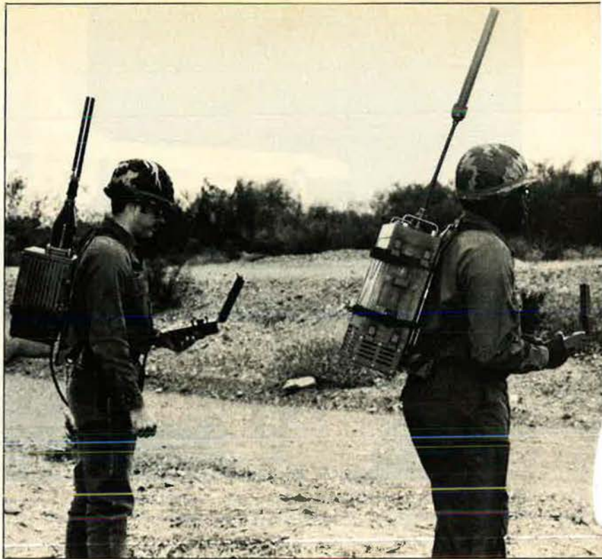
Navstar navigation aids being field-tested at the Yuma Proving Grounds in Arizona. Weighing twenty-seven pounds in backpacks, the equipment receives signals from orbiting satellites to determine ground location within thirty feet. Sponsored by USAF's Space and Missile Systems Organization, Navstar equipment is being developed for all the services. Nine NATO nations are interested.
