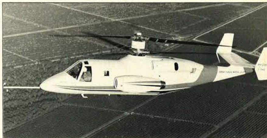
This Sikorsky Advancing Blade Concept (ABC) research helicopter recently achieved 165 knots during high-speed flight tests being conducted at the Sikorsky facility near West Palm Beach, Fla. The program's goal is a speed of 300 knots. A feature of the aircraft is two outboard-mounted Pratt & Whitney J60 turbojet engines for auxiliary thrust. The ABC system consists of two counterrotating blades mounted on a single shaft, eliminating the conventional tail rotor and providing "greater maneuverability and improved hover efficiency over conventional rotary-wing aircraft," the company said. Further, the ABC system "effectively combines the vertical lift and low-speed flight efficiency of the helicopter with the forward high-speed flight efficiency of fixed-wing aircraft."
