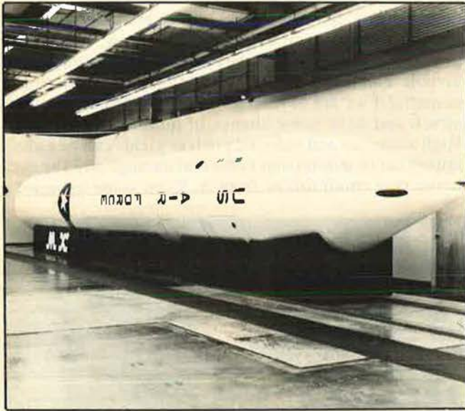
MX in a survivable basing mode is the "most important program we have in the Department of Defense," according to General Jones. The photo shows an MX mockup with a ninety-two-inch diameter and a seventy-two-foot length.
