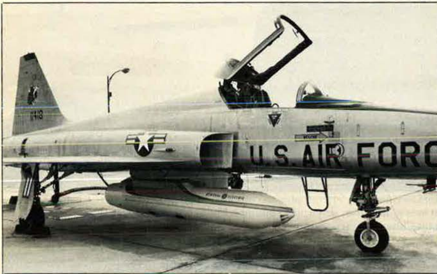
Flight testing of this 30-mm gun pod is currently taking place aboard a Northrop F-5E at Edwards AFB, Calif. The GE-developed gun pod is designed to give the F-5E added firepower on air-to-ground missions, especially against tanks. The pod weighs less and is slightly smaller than the standard 275-gallon centerline fuel tank. The gun can fire at the rate of 2,400 rounds per minute.
