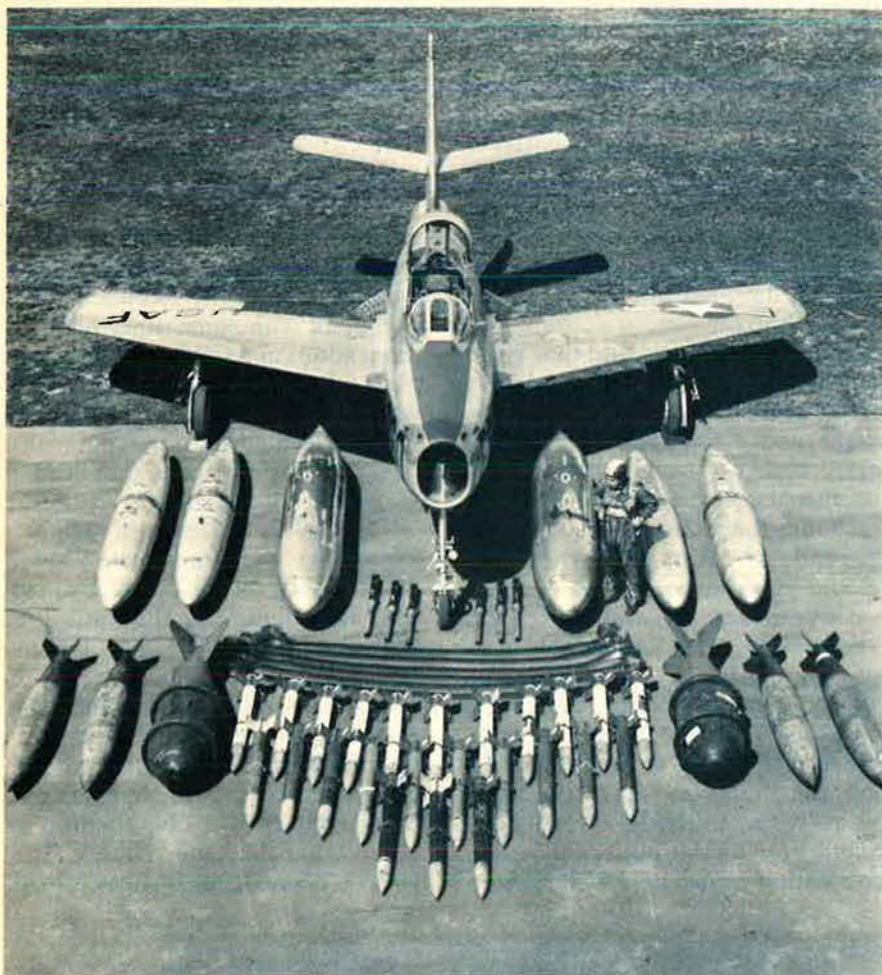
The F-84F could deliver various combinations of the bombs and rockets shown in the front row, or nuclear weapons using over-the-shoulder techniques. Its range could be extended by aerial refueling or by using the tanks shown above.
