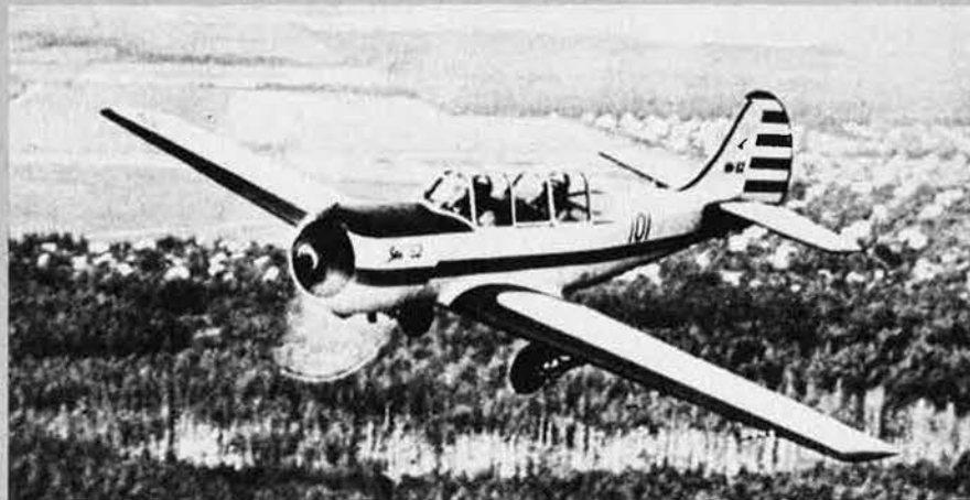
The semi-retractable landing gear of the Yak-52 is well shown in this photograph
