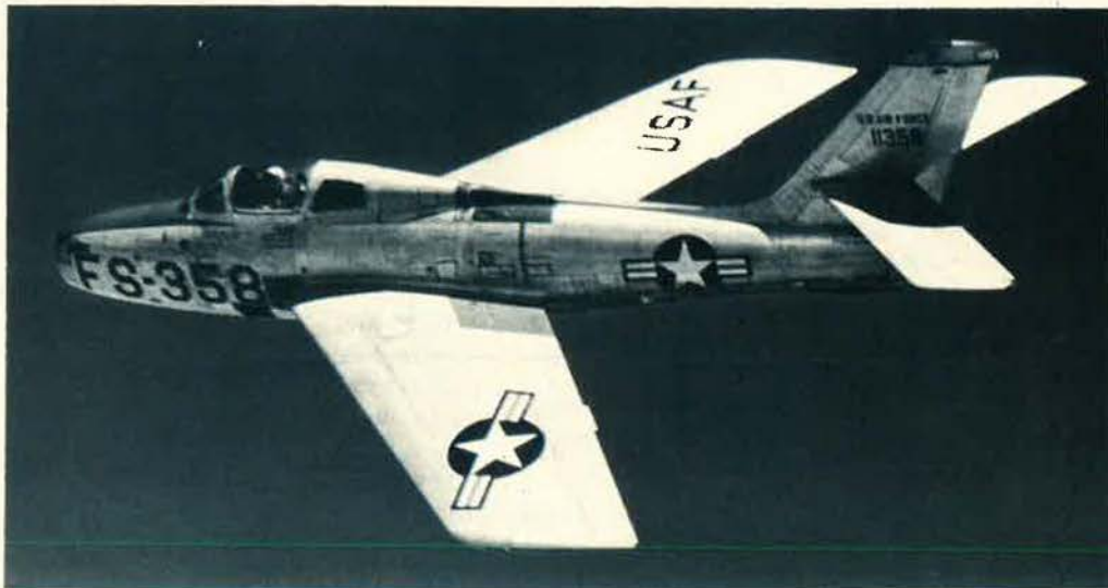
Delivery of F-84Fs to both TAC and SAC began in 1954. The F had six .50 guns and could carry 6,000 pounds of ordnance. Some 1,300 were produced for NATO allies; the ANG flew the F until 1971.
