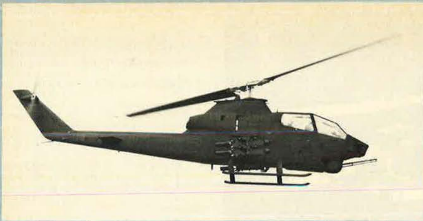
AH-1S version of the single-engined Bell Model 209 HueyCobra, with TOW missile launchers
