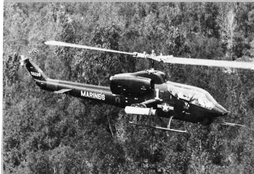
Bell AH-1T, improved version of the twin-engined SeaCobra for the US Marine Corps
