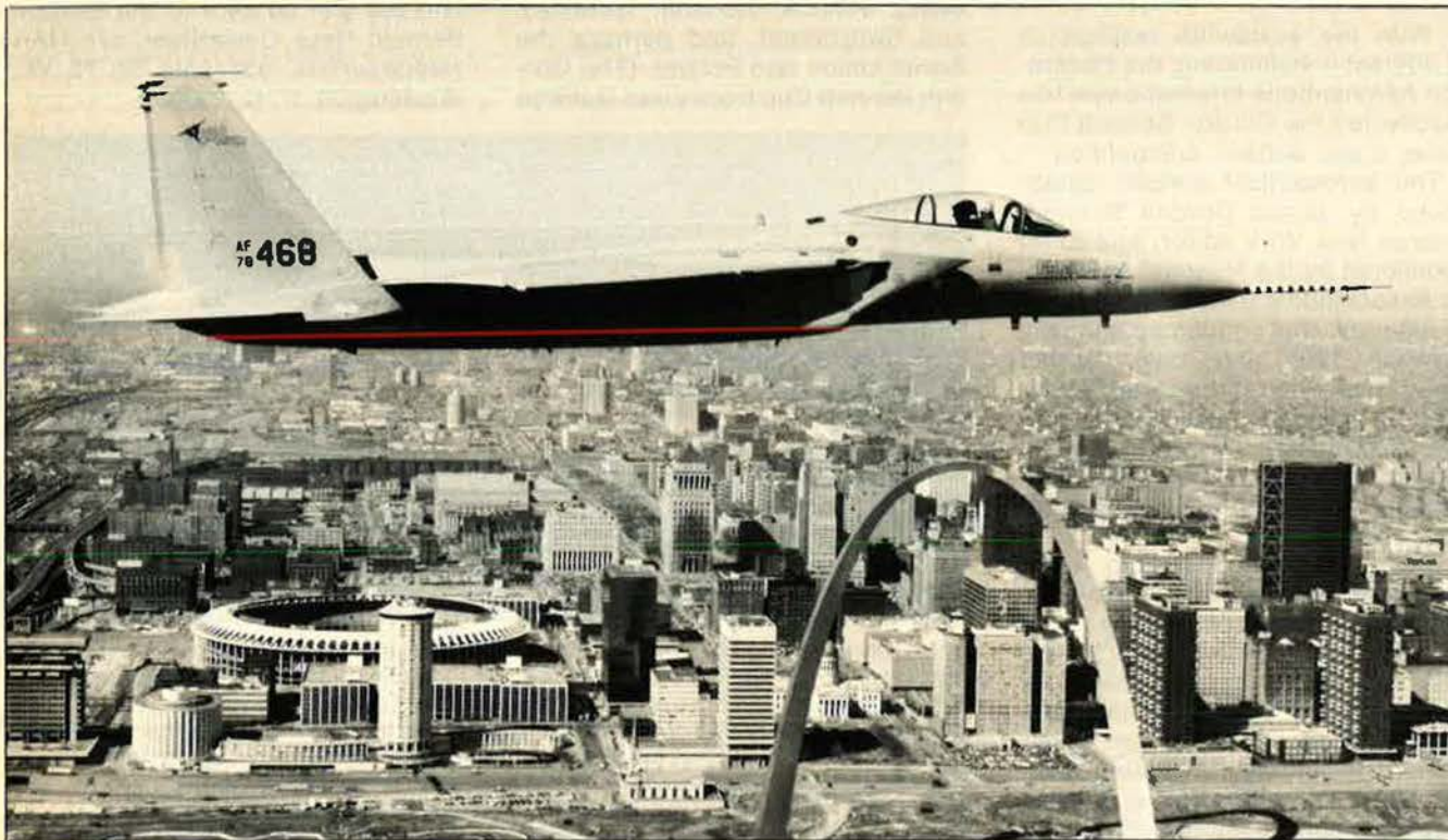
The first "C" version of the F-15 Eagle, with twenty percent more internal fuel capacity plus fittings for FAST Pack conformal fuel pallets, flew in late February at McDonnell Douglas Corp.'s McDonnell Aircraft division in St. Louis.
