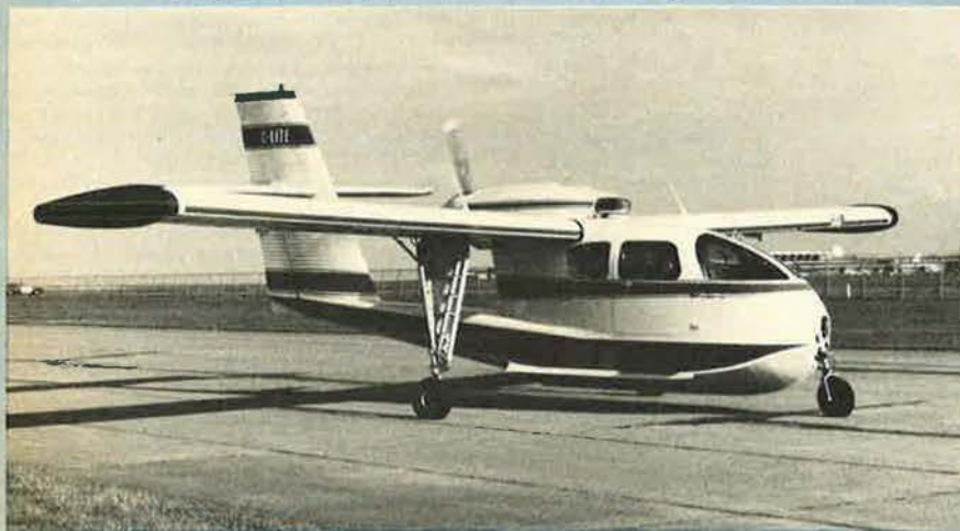
Trident TR-1 Trigull prototype, with wingtip floats retracted
