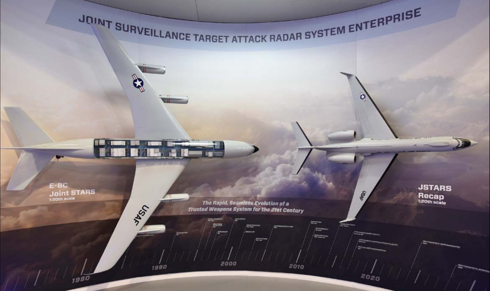
Northrop Grumman models illustrated its proposal for shrinking JSTARS to fit on a Gulfstream 550.
