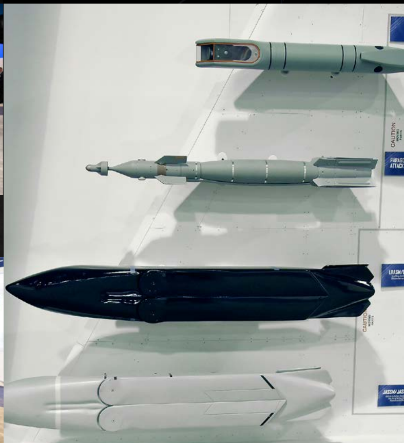
A generic fighter aircraft wing bears (from top) Lockheed Martin's Sniper targeting pod, Paragon guided bomb, and the LRASM and the JASSM stealth anti-ship/land-attack missiles.
