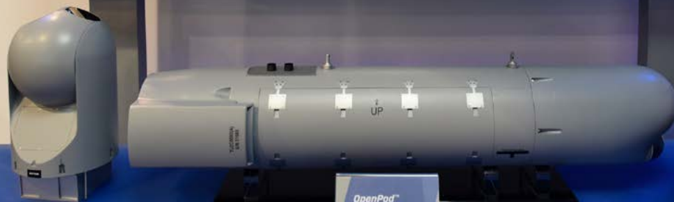
With real estate on combat aircraft hardpoints growing increasingly precious, Northrop Grumman showed the Open Pod, an open-system architecture, reconfigurable system of sensors. The first version will include infrared search and track and targeting devices.
