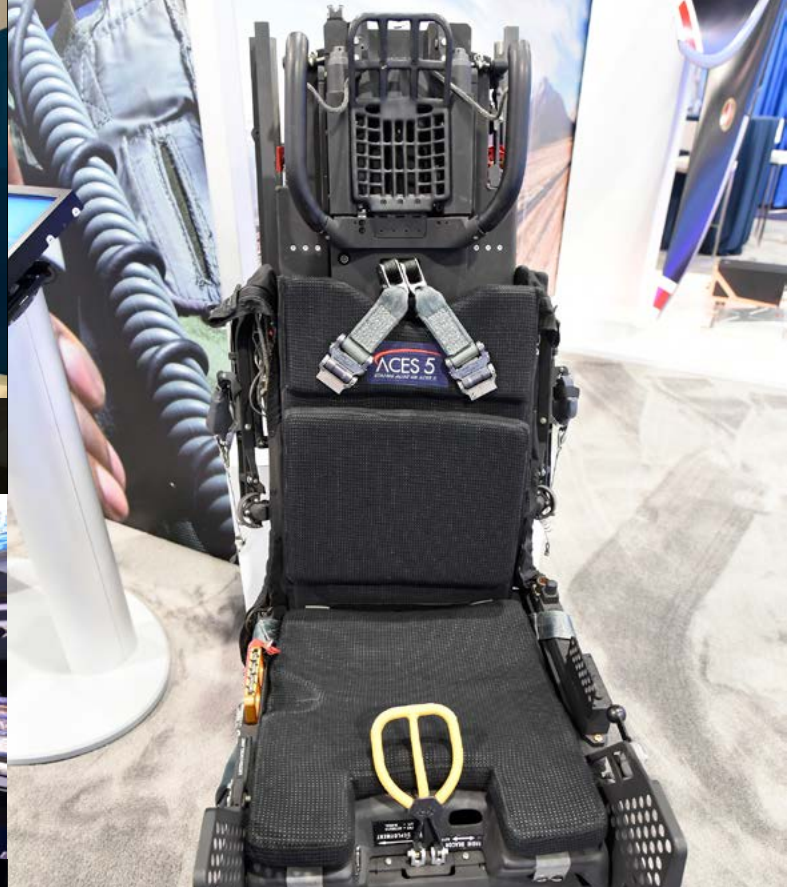
The ACES 5 is UTC Aerospace System's latest generation of the combat aircraft ejection seat.
