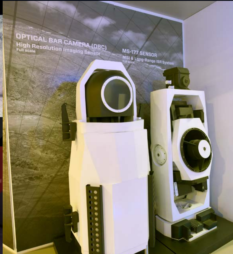
Modular payloads for Northrop Grumman's Global Hawk surveillance aircraft were shown in these full-scale models of the Optical Bar Camera (left) and MS-177 multispectral sensor.
