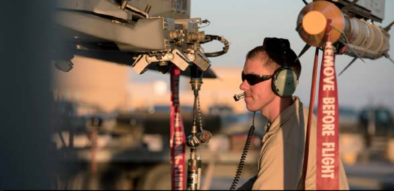
TSgt. Joseph Benoit tests the functionality of a weapons rack on an F-16. Photo: MSgt. Benjamin Wilson
