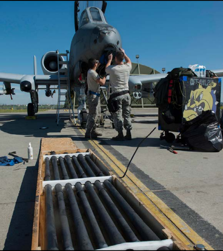
SSgt. Stephens Doherty (left), and SrA. Nathaniel Awrey reassemble the GAU-8/A rotary cannon on an A-10 at Incirlik. Photo: A1C Devin Rumbaugh
