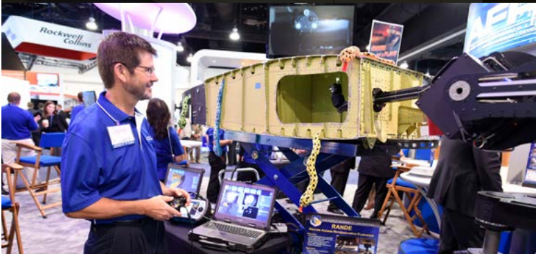
Charles Buynak of the Air Force Research Laboratory demonstrates a snake-like robot that can inspect parts of an airplane where tech crews can't go.
