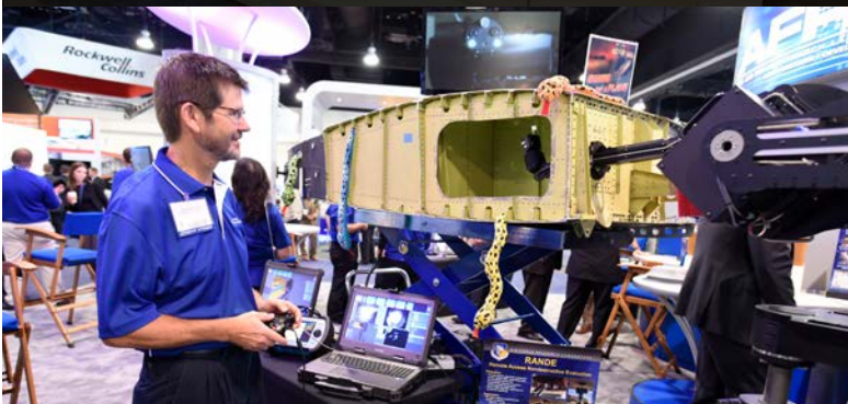
Charles Buynak of the Air Force Research Laboratory demonstrates a snake-like robot that can inspect parts of an airplane where tech crews can't go.
