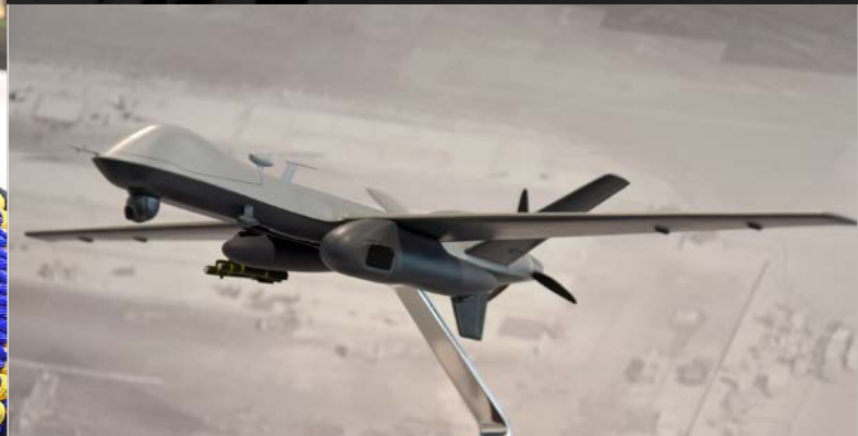
This General Atomics MQ-9 Reaper model carries an MS-110 multispectral recce pod made by UTC Aerospace Systems.
