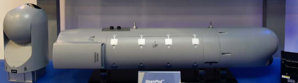
With real estate on combat aircraft hardpoints growing increasingly precious, Northrop Grumman showed the Open Pod, an open-system architecture, reconfigurable system of sensors. The first version will include infrared search and track and targeting devices.
