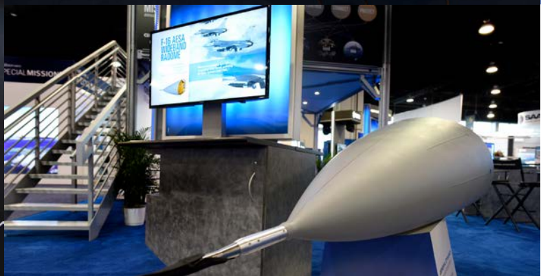
An active electronically scanned array radar needs a new radome. At its booth, General Dynamics showed off this one for an F-16.
