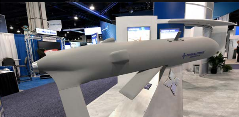
This full-size "Gremlin" by General Atomics Aeronautical Systems is one proposal for a class of remotely piloted aircraft cheap enough to be sacrificed if necessary.
