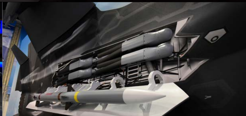
Raytheon packed a model of the F-35 fighter with its AIM-120 AMRAAM radar-guided dogfight missile and a hefty load of Small Diameter Bomb IIs.
