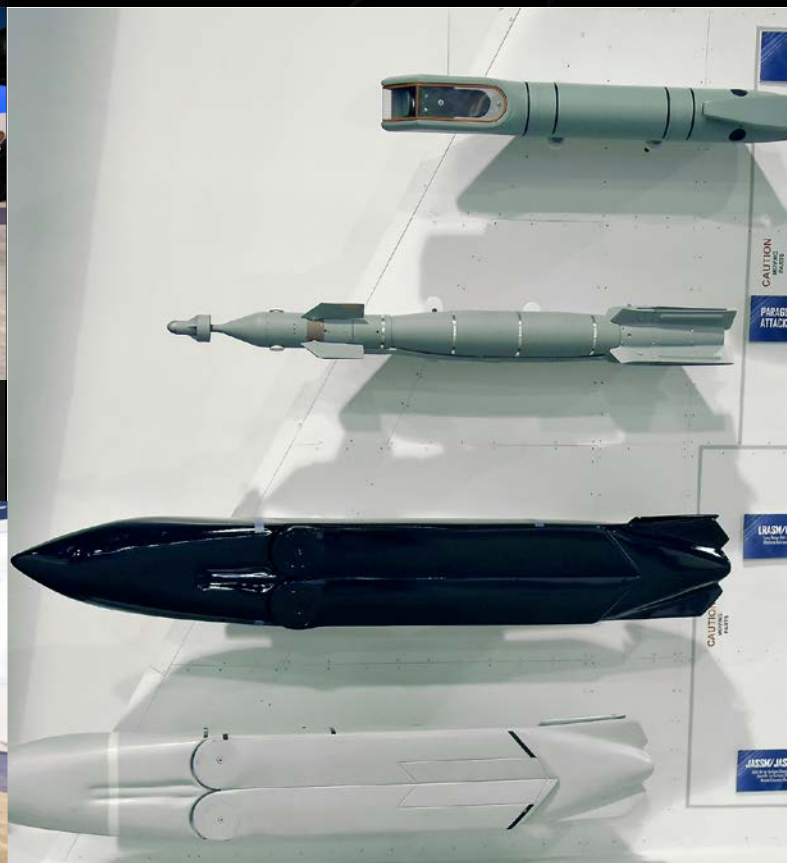
A generic fighter aircraft wing bears (from top) Lockheed Martin's Sniper targeting pod, Paragon guided bomb, and the LRASM and the JASSM stealth anti-ship/land-attack missiles.
