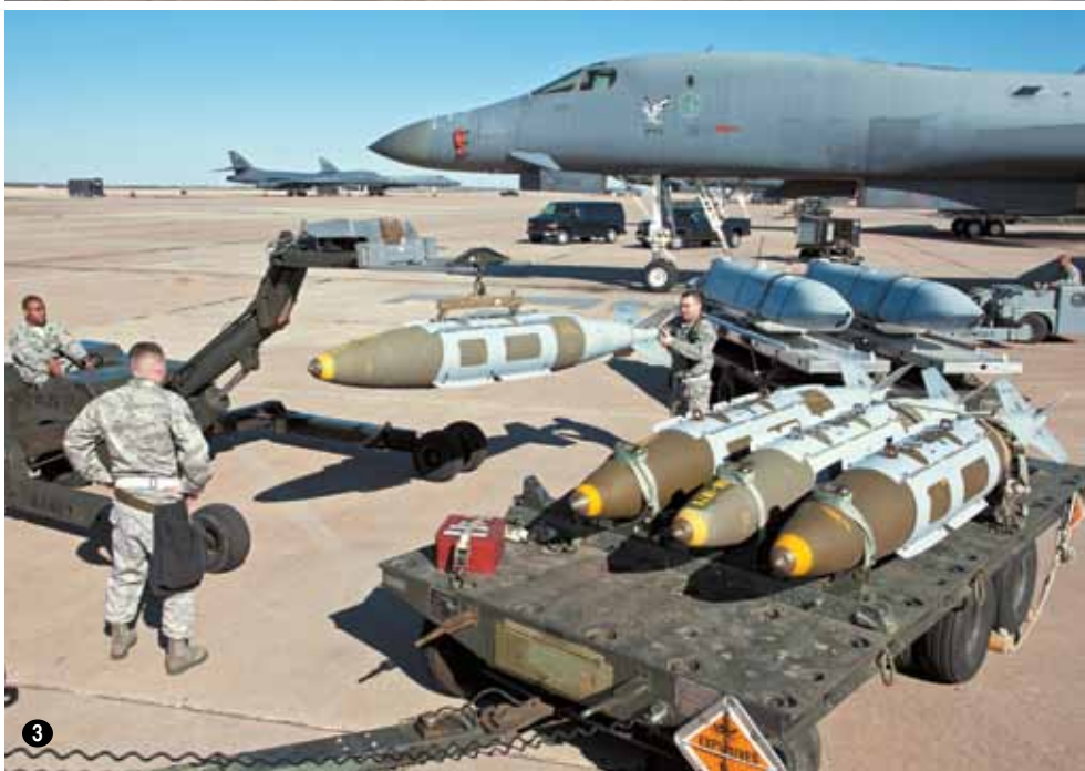
11 Capt. David Grasso demonstrates the Bone's power and agility, making a near-vertical climb over Texas in 2011. 12 A B-1B cruises over the New Mexico desert. 13 Taylor lifts a JDAM with a jammer as Rose (c) and Garza prepare to load the satellite guided bomb into a weapons bay. 14 The view from the cockpit as another Lancer lines up on the runway for takeoff.
