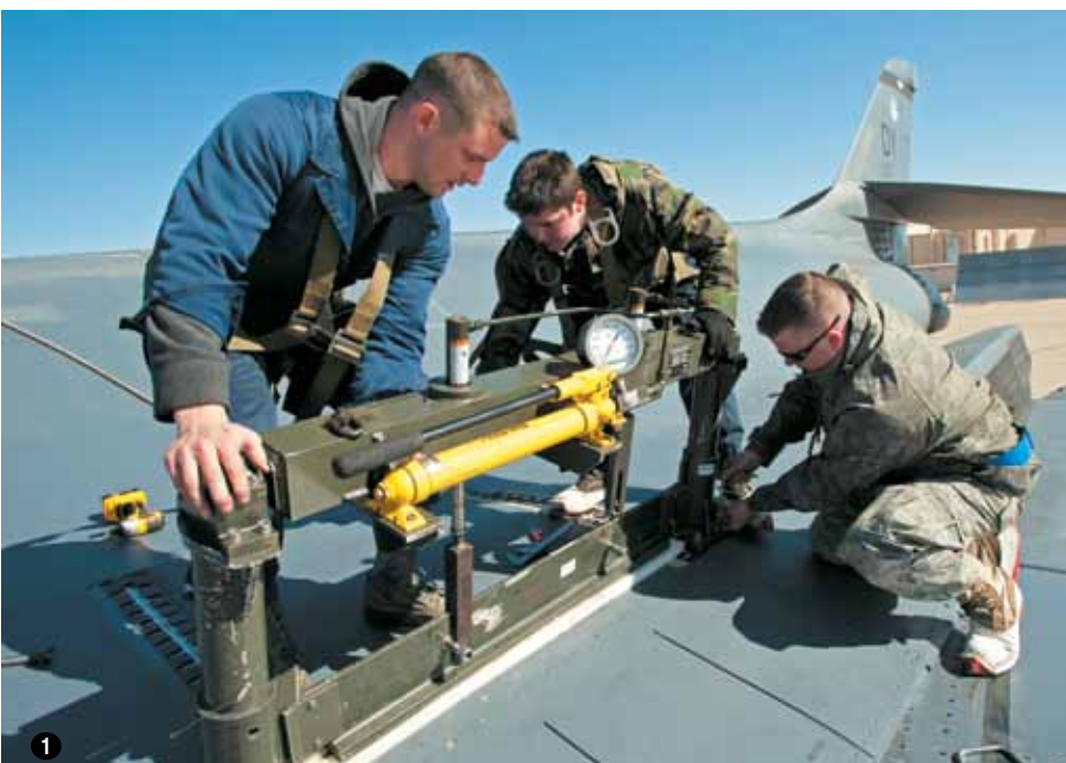
111 (l-r) SrA. Jason Crane, A1C Jeremiah Jansen, and SSgt. Scott James, crew chiefs at Dyess, work on a B-1's wing carry-through spring panel. The aircraft has variable-geometry wings and employs its forward wing setting for takeoff, landing, air refueling, and some high-altitude weapons scenarios. For combat and high subsonic or supersonic flight, it uses the aft wing sweep configuration. 121 A 9th Bomb Squadron B-1 takes to the sky on a training mission from Dyess. The 7th Bomb Wing hosts the Air Force's only B-1 formal training unit.
