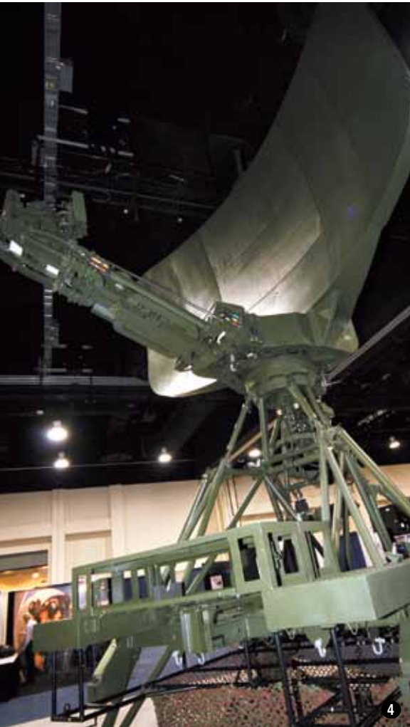
13 Goodrich's booth emphasized sensors and intelligence, surveillance, and reconnaissance products. 14 Lockheed Martin erected a full-size TPS-79 Expeditionary Air Surveillance Radar in the exhibit hall. It can be operated from a mobile shelter or a remote site. Ample space in the exhibit hall makes possible large displays such as this.
