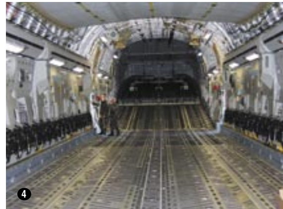
[4] The capacious C-17 cargo bay, 88 feet long, 18 feet wide, and 12 feet high, can carry 170,900 pounds of cargo. It's carried everything from helicopters to an elephant, and is able to land in just a few hundred feet—a capability unique to USAF. ■
