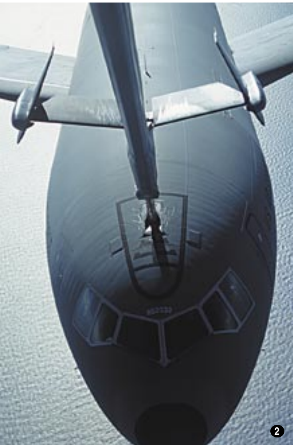
[1] TSgt. Chrissie Valenza and SrA. Simon Hunt check the radar and other avionics in a C-17's nose. Both are with the 305th Maintenance Squadron. [2] Trapezoidal markings on USAF aircraft assist boomers in locating and plugging into refueling receptacles. This one is on a KC-10.
