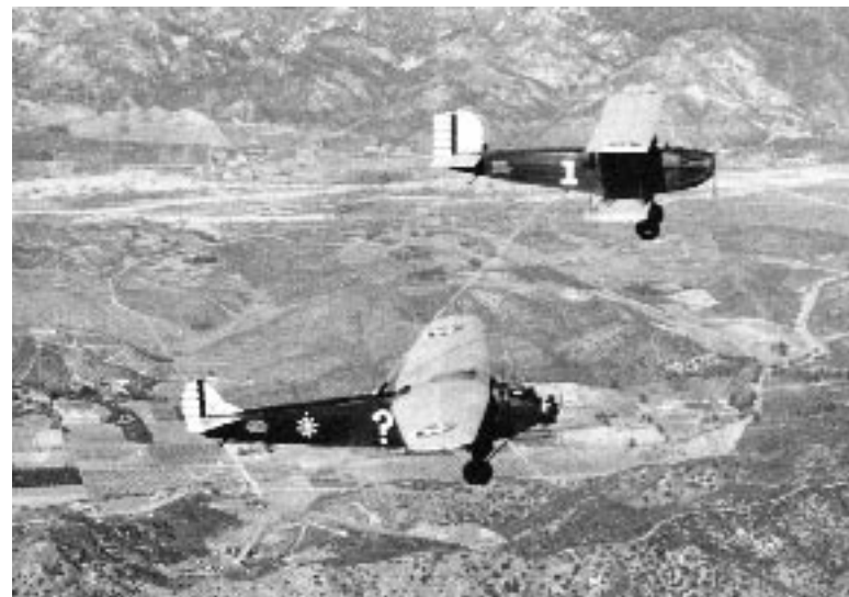
The Air Corps' Fokker C-2 Question Mark (lower) takes on fuel during its Jan. 1-7, 1929 record endurance flight.
