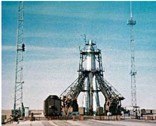
Left: Illinois newspaper covers the local "beep" phenomenon. Above: R7 booster (number 8K71PS) hours before blastoff. The R7 began life as an ICBM, but achieved its greatest fame as a launch vehicle.
