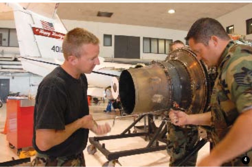
[2] The top missions of the MQ-1 (here returning to an airfield in Afghanistan) are interdiction and armed reconnaissance against critical and fleeting targets. [3] Four antenna, or "bird slicers," in front of the canopy glass were part of the F-16's IFF avionics. [4] Two 119th Wing airmen, TSgt. Charles Welle and SSgt. Mathew Andvik, swap out a C-21 engine.
