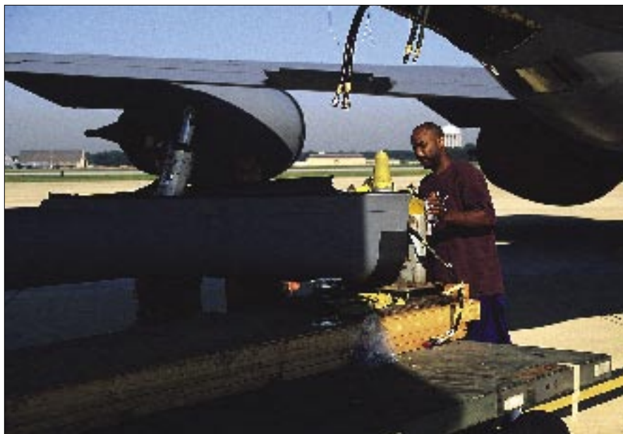
At left, MSgt. Zerrik King, a Reservist with the 459th ARW, works to reinstall a newly serviced boom onto one of the unit's KC-135s at Andrews AFB, Md. The high-speed boom can transfer fuel at a rate of up to 6,500 pounds per minute.
