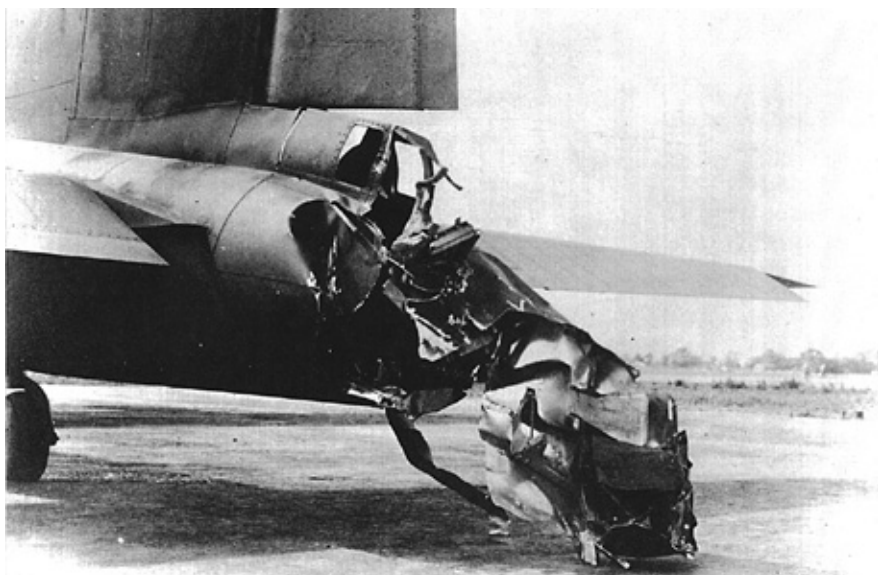
Left: The tail gunner's compartment of this B-17 nearly has been ripped away from the aircraft. This was an unfortunate fratricide incident: The damage was caused by a falling bomb.
