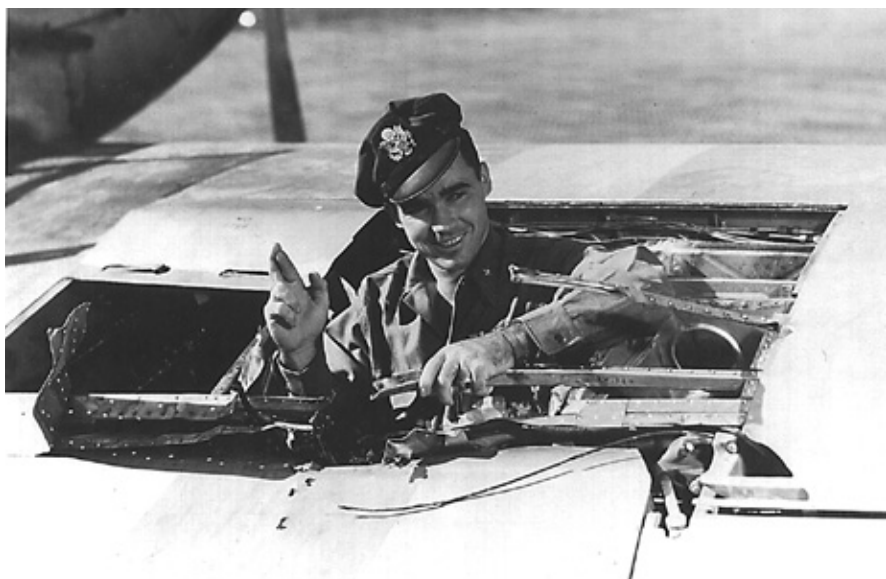
Above, this B-26 Marauder landed hard in England in September 1943 after flak had hit its landing gear lock.
