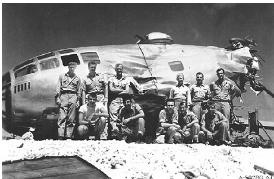
On Saipan in the Pacific, Capt. James Pearson and his crew line up before what is left of their B-29. The fuselage at left was actually lucky to be in such "good shape." After a mission over Tokyo, this bomber returned 1,500 miles through bad weather with both engines out on one side and with the fuselage torn open by a runaway prop. Finally, the nose was completely torn off in the aircraft's crash-landing.
