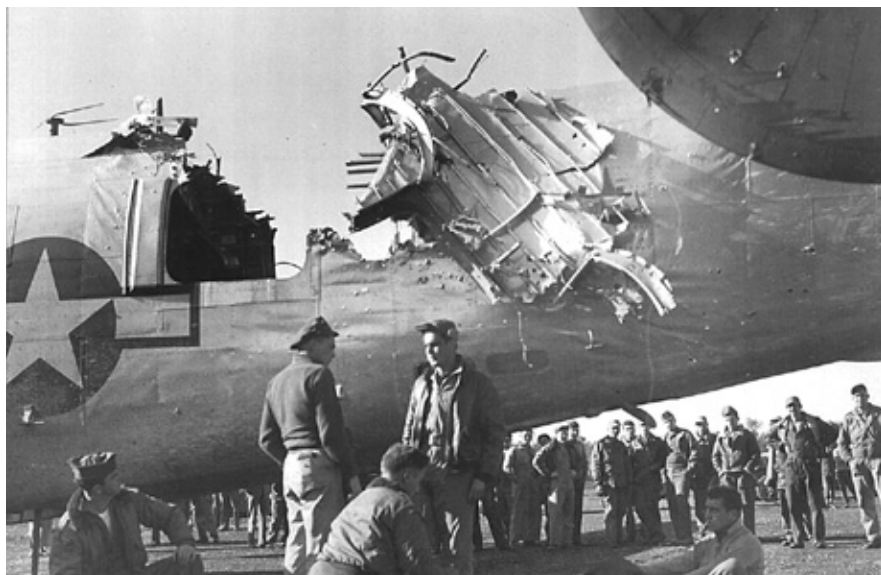
A flak shell pierced the bottom of this B-24 at right—but the shell didn't detonate until it struck the top of the bomber's waist section. Besides killing a crew member, the exploding round blew the top of the mid-section away, severing the aircraft's rudder cables.
