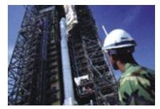
At top, the mobile service tower has been pulled back, leaving the launch vehicle in full view. Moving the million-pound tower without damaging the rocket requires extreme care. Above, MSgt. Lou Moyer, noncommissioned officer in charge of the 3rd SLS's booster section, observes as the door to the tower is prepared for rollback.
