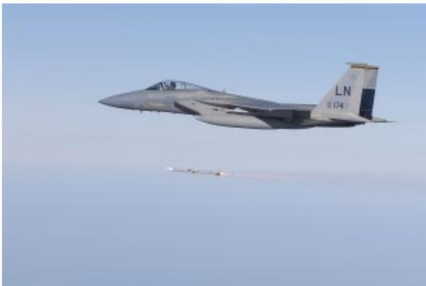
At left, an F-15C pilot from Lakenheath launches an AIM-120A AMRAAM at a subscale drone during a live weapons-fire event.
