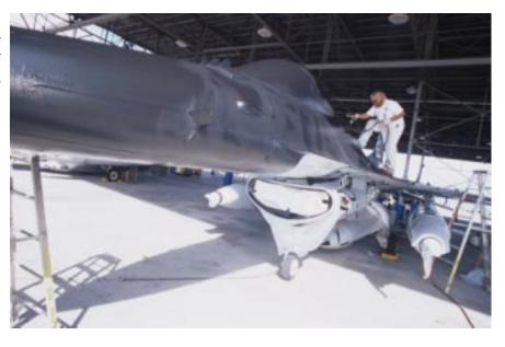
At left, AMARC aircraft preservation technician Manny Vasquez applies a coat of Spraylat to an F-16. Aircraft arriving at the facility go first to this long open shelter. Workers drain all fluids and begin the process that will preserve the fighter. Storage is customized for three different types of use—a return to flying, spare parts, or eventual disposal. In all cases, the ejection seat system is deactivated and aircraft seams are taped over.
