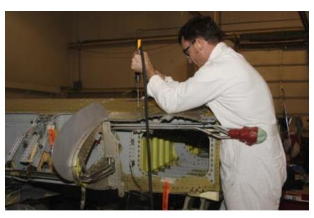
The facility completed its first A-10 SLEP wings in 2003. At present, it takes about 140 days to complete a set. Each wing has its own individual quirks and problems; many of the repairs are "handmade" in nature.
