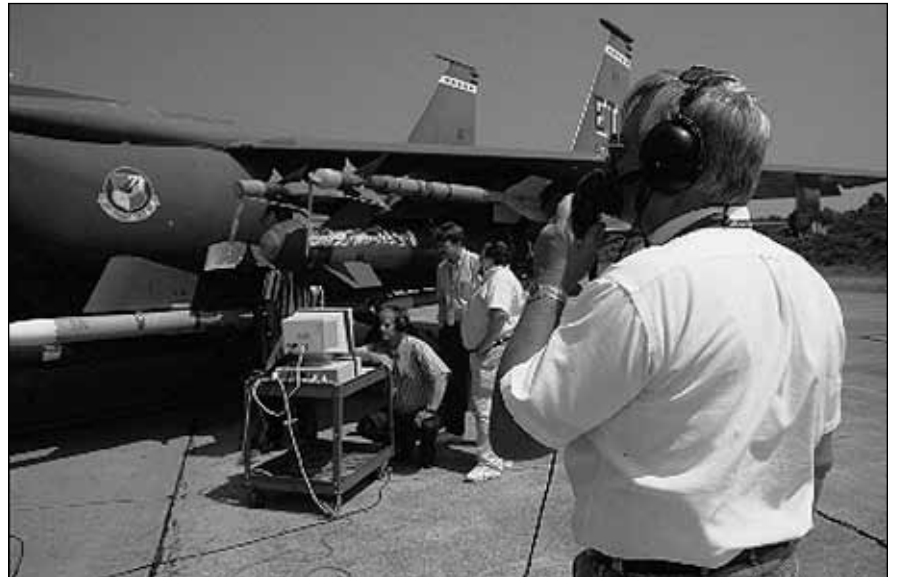
Company and program technicians at the side of the airplane conduct comprehensive checks and rechecks. A computer strapped to a cart becomes an impromptu mobile test set as technicians labor to ensure that the GBU is "talking" to the aircraft and that both are feeding data to the pods. With only 45 days to get the weapon into service, every flight was critical.
