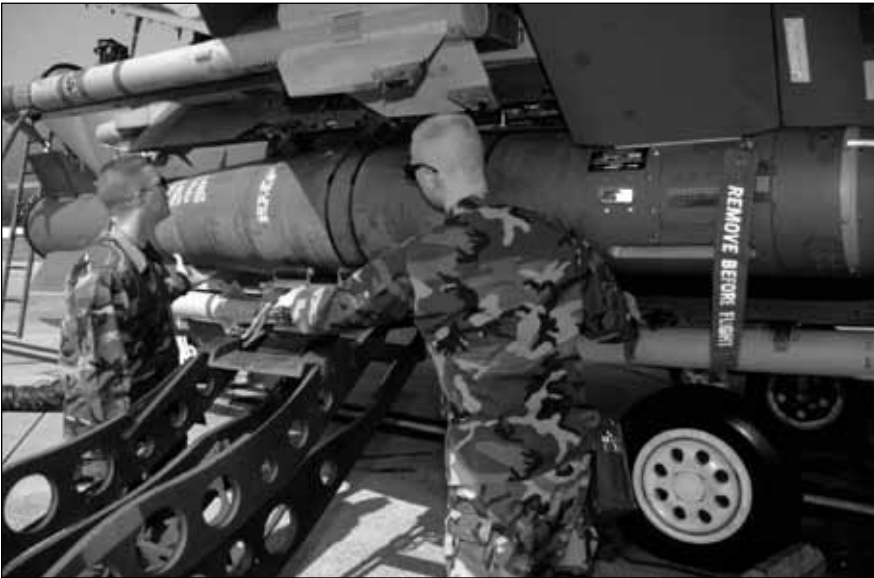
A1C Richard Kleen (left) and SSgt. David Currie carefully position the weapon on an F-15E for the drop test. Everything must be right to ensure that a test subject is not accidentally lost. Below, a tech rep positions cameras that will record every instant, at every angle, of the release.
