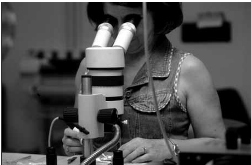
Above, Carlotta Garrett uses a microscope to fine-tune the circuitry of a GPS-equipped GBU-15, while Honeywell technician Ken Bett (at left) carefully wraps the circuits in foil prior to the test to help keep them cool and help ensure the data obtained are accurate.
