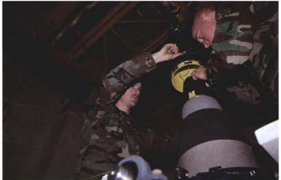
Like the rest of the missile, the warheads themselves are periodically checked and maintained. At F. E. Warren, SSgt. Gary J. Skowronek, reentry vehicle maintenance team chief, goes by the book in overseeing the replacement of the last of up to 10 independently targetable reentry vehicles for the business end of an LGM-118A Peacekeeper missile. The Peacekeeper, fully operational since 1988, is larger, heavier, and more accurate than the Minuteman. The Styrofoam ring around one of the reentry vehicles protects it and also serves as a place for technicians to place their tools temporarily. At right, SrA. Kelly Summerfield and SrA. Mark Poani (right) carefully replace the cap on a reentry vehicle. Below, on the Minuteman III side of the base's weapons facility, SrA. Corey LaRock and SrA. James Callari (right) check the forward component of the reentry system.
