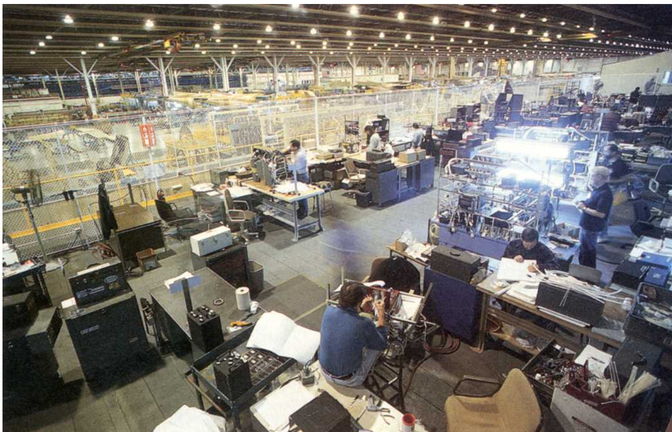
In a compact section overlooking the 3.5-million-square-foot main assembly area, electronics technicians assemble, check, and install wiring bundles to some of the avionics boxes for later installation on the floor below. At right, Freda M. Wingard and other workers install some of the wiring in the cockpit subassembly. This requires squeezing into some tight corners where even a future crew chief will never have to go. Nearly 9,700 people work at this Marietta plant, more than 6,000 of them in the Hercules program.
