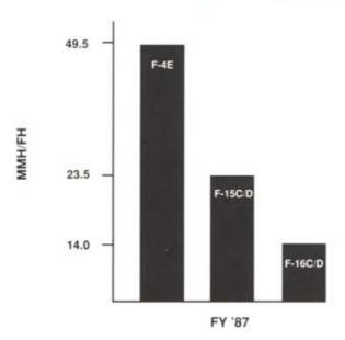
This chart demonstrates that the latest model F-16C/D aircraft is not only less likely to break than other aircraft but is also easier to maintain and repair—almost two times easier than is the case with the F-15C/D and more than three times easier than is the case with the F-4E. Result: lower personnel cost, more efficient use of manpower, and higher aircraft availability.
