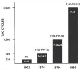
Today's modern engines require proportionally fewer hot section overhauls than their predecessors. This chart demonstrates hot section overhauls per given number of "tac cycles." (A tac cycle refers to a sequence an engine goes through—for example, "idle" to "military power without afterburner.") It is a key measure of engine performance under stress. Engines in F-15s show a tenfold improvement over those in F-4s. Maintenance needs and downtime for the aircraft are lower.
