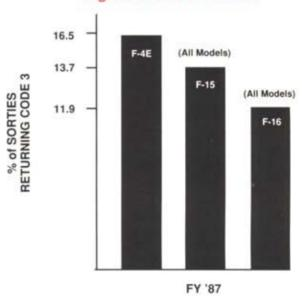
This chart shows the comparative break rates for certain fighter aircraft systems. "Code 3" means a serious system failure that prevents the aircraft from flying until it is fixed. (Code 1 means all systems function properly; Code 2 means a malfunction that does not have to be fixed right away.) F-16 and F-15 reliability stands significantly higher than that of the earlier generation F-4. F-16s, thus, spend less time in the shop and more in the air.
