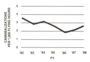
This chart shows the cannibalizations per 1,000 flying hours for aggregate USAF aircraft. "Cannibalization" means stripping a temporarily out-of-service aircraft of parts in order to keep other aircraft flying. The practice is the prime cause of "hangar-queen" aircraft. After a steep decline throughout the 1980s, the rate has turned up—principally due to spares being in tight supply.
