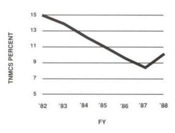
This chart shows the percentage of aggregate USAF aircraft rated total not mission-capable supply (TNMCS). TNMCS means that one or more parts are missing from the aircraft and that therefore the aircraft cannot perform its mission. From FY '82 to FY '87, the percentage of TNMCS was cut nearly in half. Now, however, It is edging upward. The situation today remains much improved over that of the early 1980s.
