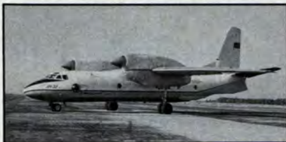
Antonov An-32 in production form, with extended overwing nacelles
