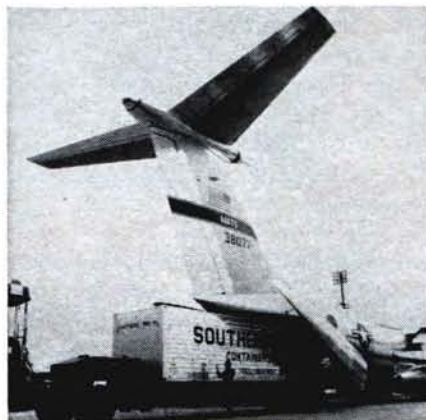
The C-141 can carry practically anything, as witness this demonstration at Lockheed-Georgia facility, in which forty-foot-long trailer van is moved directly aboard a StarLifter, using straight-in rear loading.
