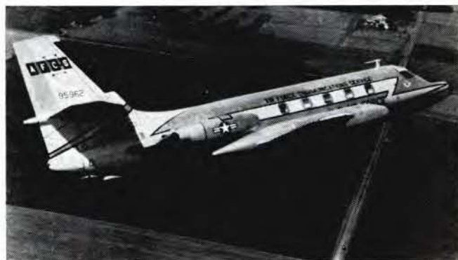
AFCS's Lockheed C-140A JetStars, specially configured for AFCS missions, are packed with electronic gear and are designed to flight-check navigational aids and air traffic control facilities set up for contingency operations.
