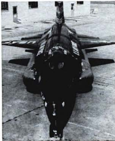
AFSC's famed X-15 rocket airplane, in cooperative efforts with NASA, has added enormous data to upper atmospheric flight knowledge. At left, improved No. 2 X-15, with two additional externally carried fuel tanks, is capable of Mach 8 speed.
