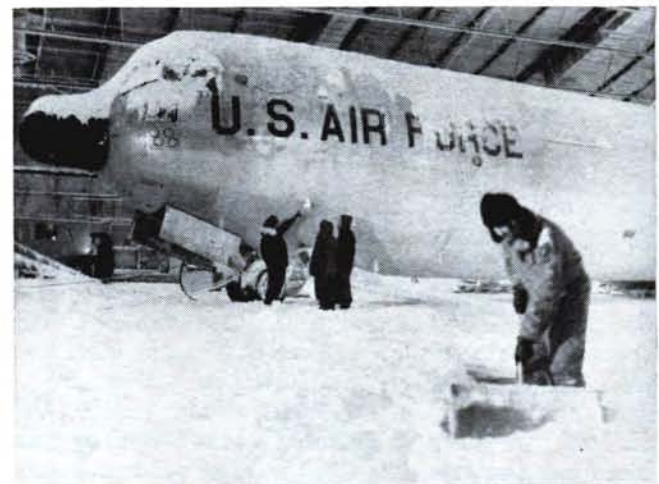
All-weather capability is increasingly essential in air operations, and Systems Command's mission includes equipment tests such as this extreme temperature study of the C-133 transport. This giant hangar at Eglin AFB, Fla., runs temperatures ranging from 65 degrees below zero Fahrenheit to 165 degrees above for its program of equipment testing.
