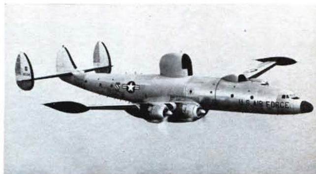
Above, the EC-121, ADC's airborne warning and patrol craft flown along East and West Coasts, serves as an extension of the nation's air defense warning system hundreds of miles seaward. The system is tied in electronically with SAGE.
