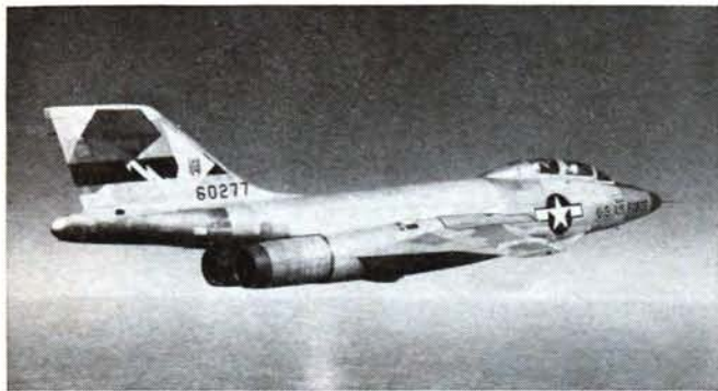
Above, ADC's supersonic McDonnell F-101B Voodoo interceptor, which joined the inventory in 1959 and carries Falcon air-to-air and Genie air-to-air missiles. Below, the Command's Convair F-106 Delta Dart, carrying same weapons, is capable of short-burst speeds of 1,500 mph plus.
